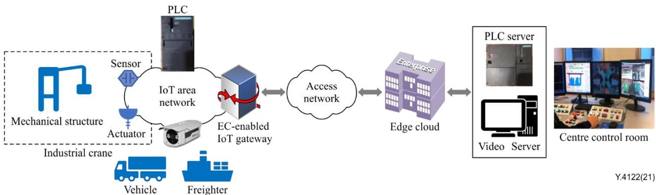
**Figure I.1 – Example of EC-enabled IoT gateway usage in crane control (PLC – programmable logic controller)**
