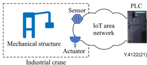
**Figure I.2 – Typical crane control before the introduction of EC-enabled gateway usage**
