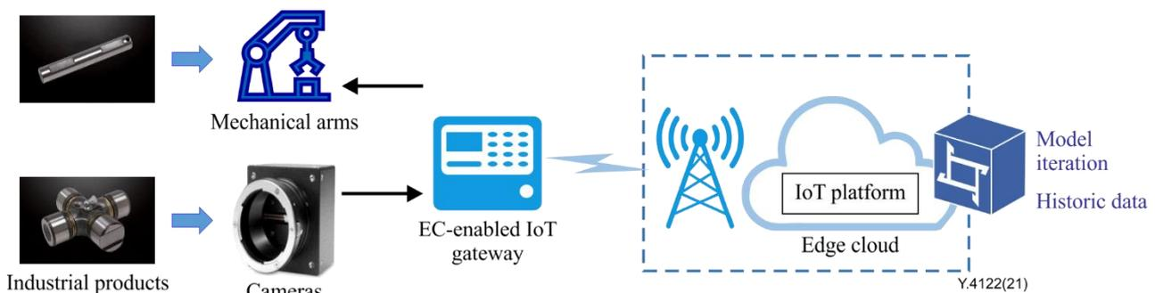
**Figure I.3 – Example of EC-enabled IoT gateway usage in product inspection**
