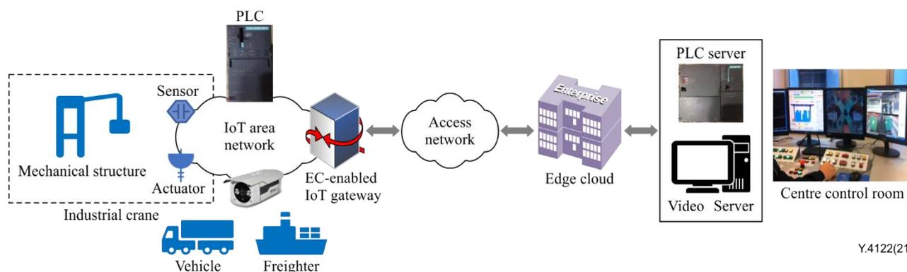
**Figure I.1 – Example of EC-enabled IoT gateway usage in crane control
