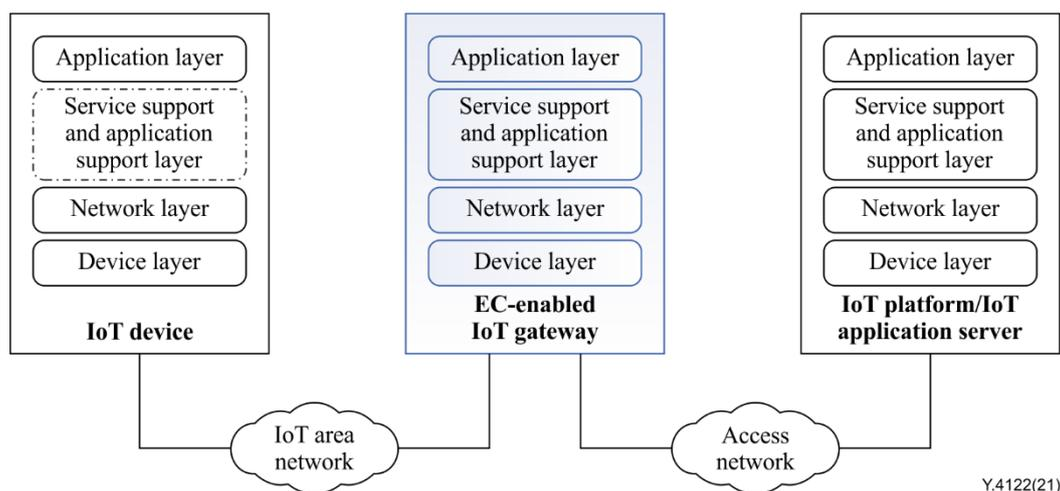
**Figure 1 – EC-enabled IoT gateway and its interworking with other IoT technical components**
