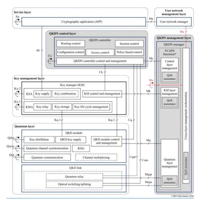
Figure 1 – Functional architecture of OoS assurance for OKDN
