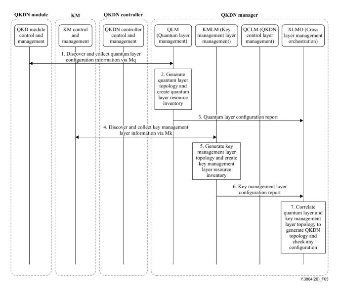
**Figure 5** – An example of configuration management procedures
