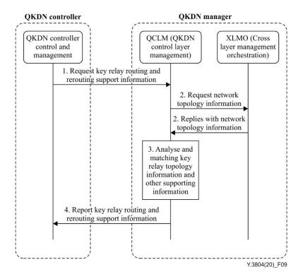
Figure 9 – An example of key relay rerouting procedures
