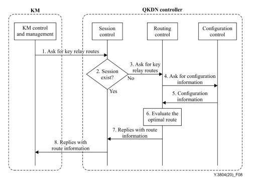
Figure 8 – An example of key relay procedures
