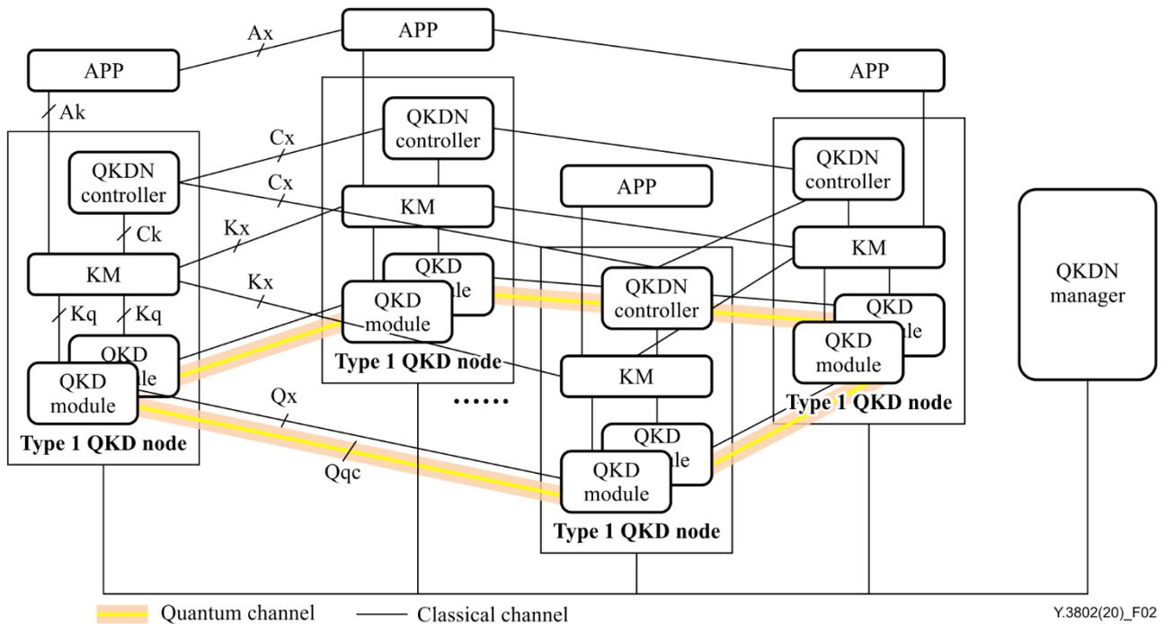
**Figure 2 – Configuration 1 of a distributed QKDN**
