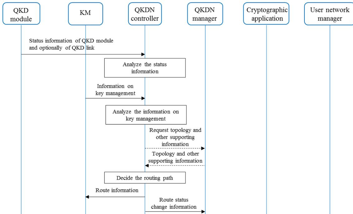
**Figure 10 – Key relay rerouting control procedure**
