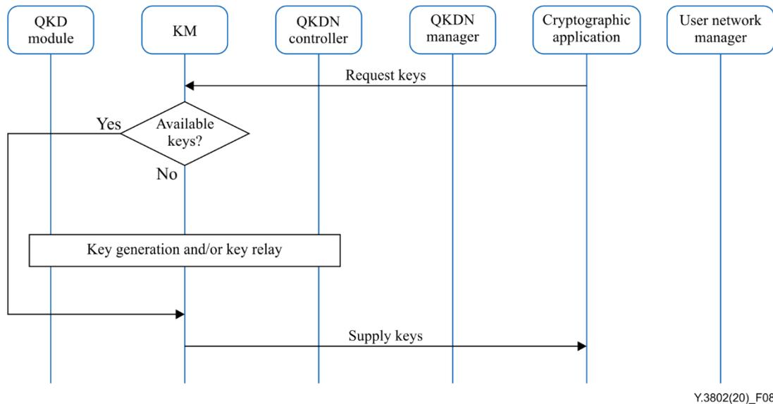
**Figure 8 – Key request and supply procedure**
