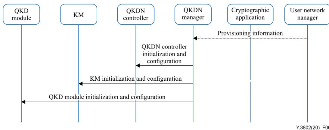
**Figure 6 – Service provisioning and system initialization procedure**
