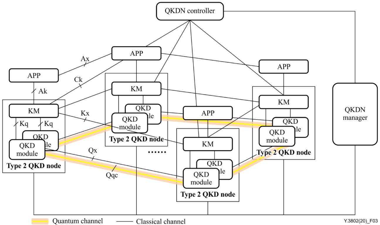
**Figure 3 – Configuration 2 of a centralized QKDN**
