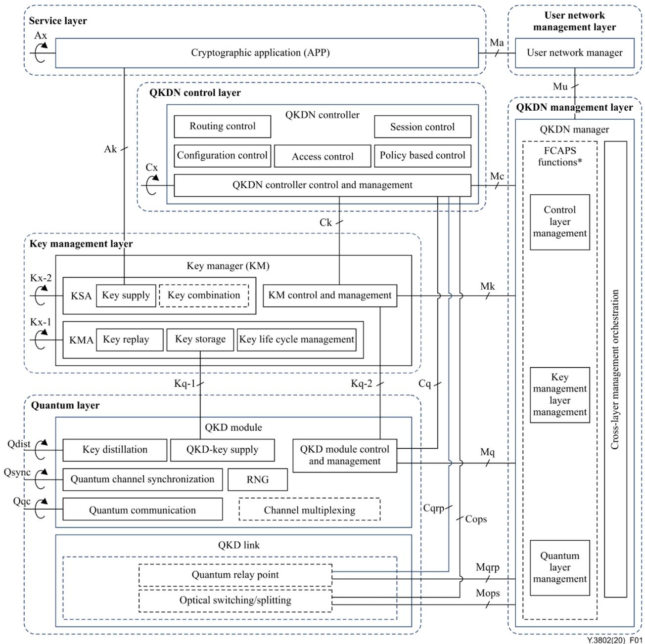
**Figure 1 – A functional architecture model of QKDN**
