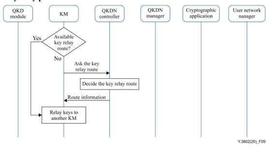
Figure 9 – Key relay procedure
