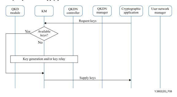
Figure 8 – Key request and supply procedure
