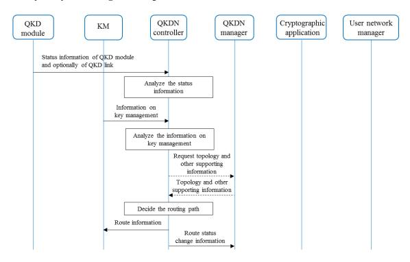
Figure 10 – Key relay rerouting control procedure
