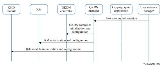
Figure 6 – Service provisioning and system initialization procedure
