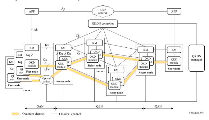
Figure 4 – Configuration 3 of a centralized QKDN with hierarchical QKD nodes
