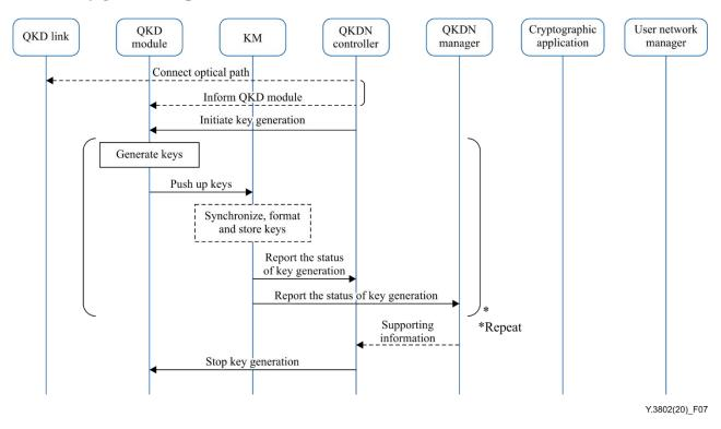
Figure 7 – Key generation procedure
