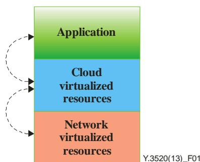
**Figure 1 – Applications residing on a single cloud computing infrastructure**
