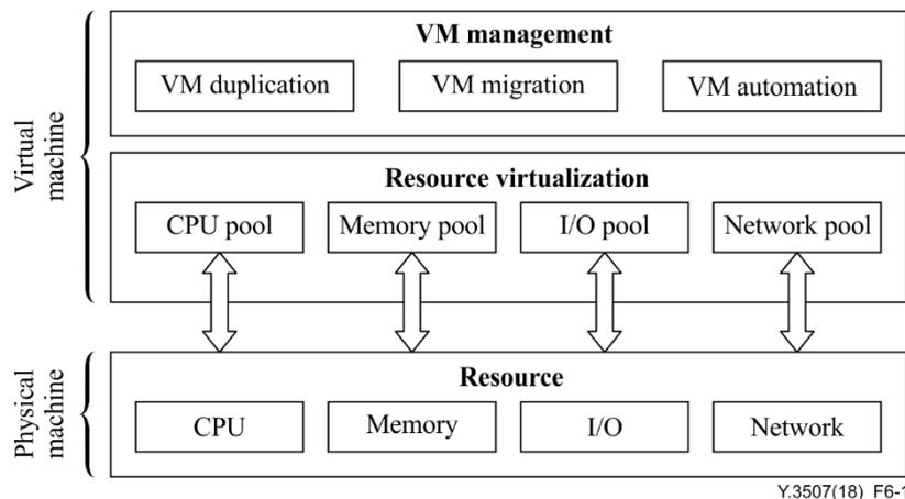
**Figure 6-1 – Concept of a computing machine in [ITU-T Y.3510]**
