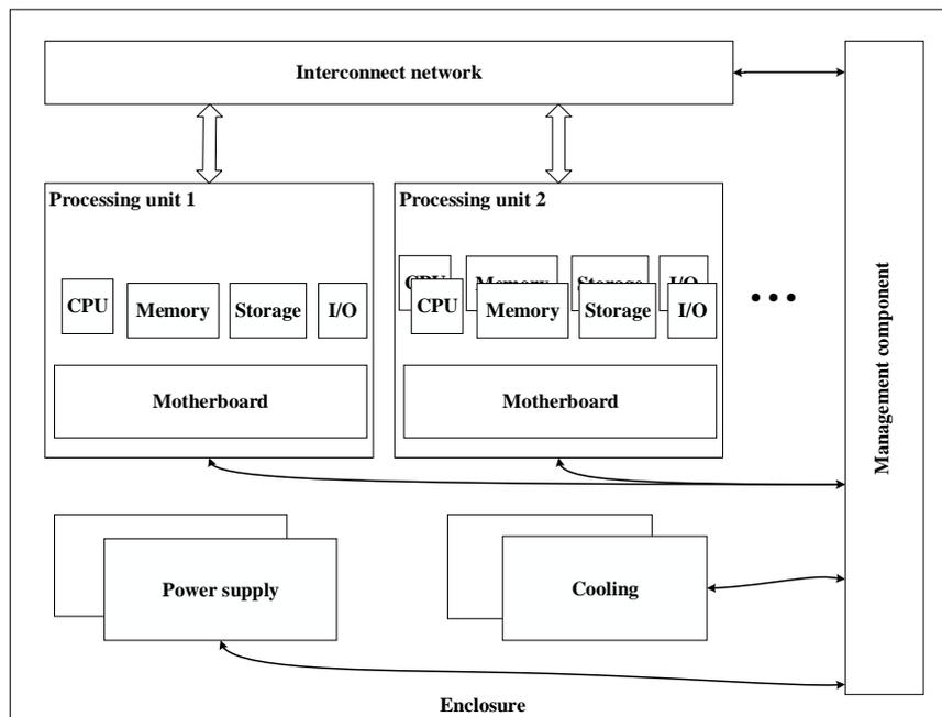
Figure 6-5 – Example of a multi-processing unit type
