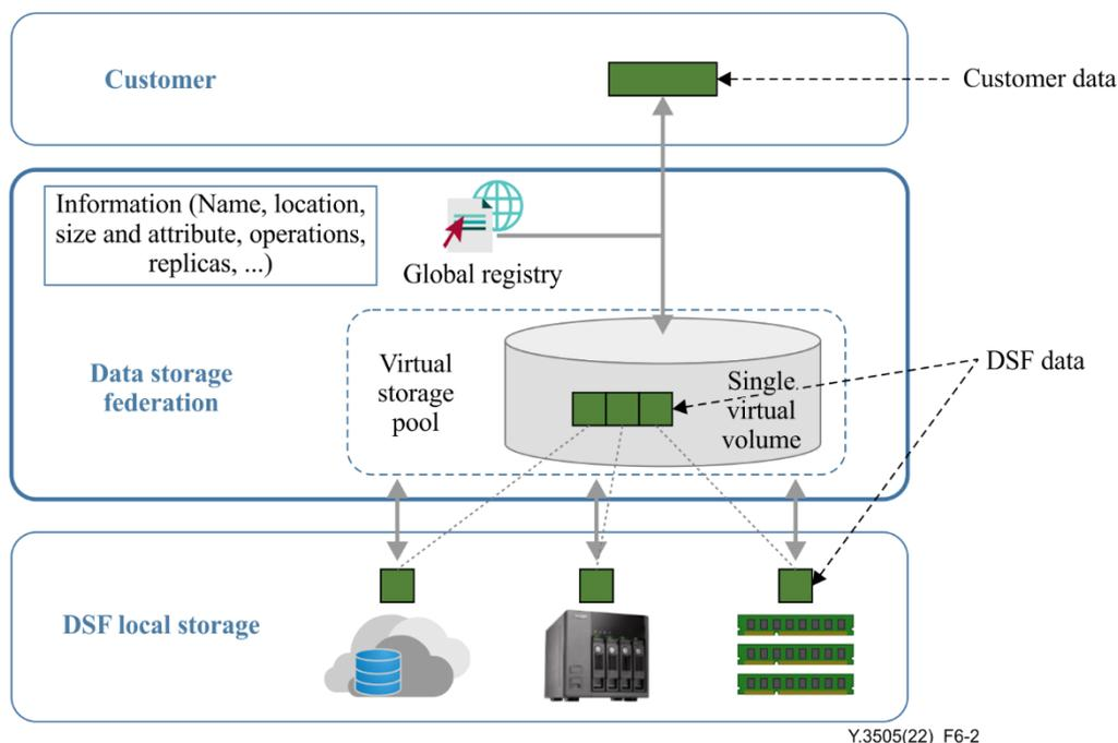
**Figure 6-2 – Example of customer data manipulation in DSF**
