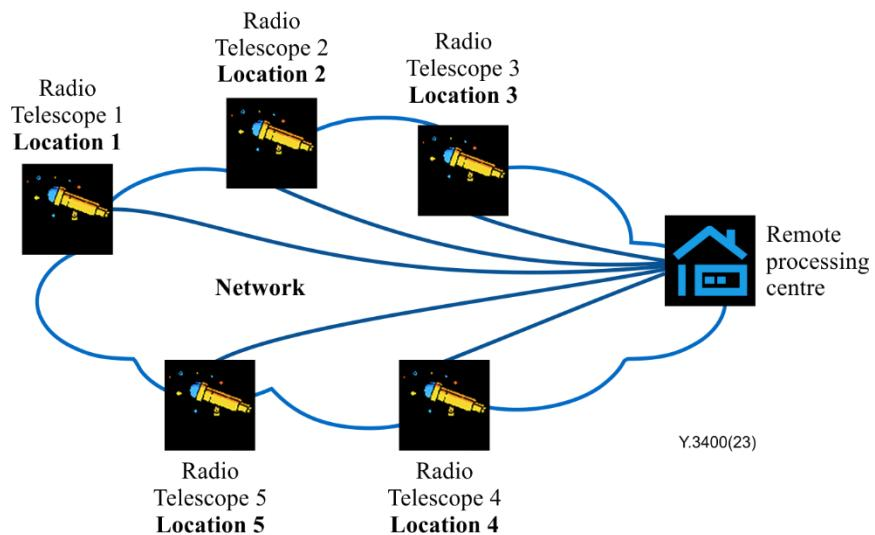
**Figure I.3 – Astronomical telescopes observation**
