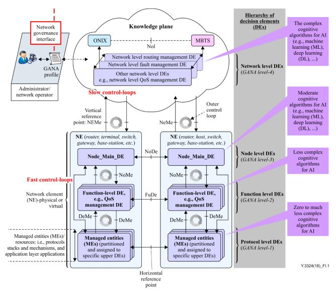
Figure I.1 – Snapshot of the GANA reference model and autonomics cognitive algorithms for artificial intelligence (AI) (Source [b-ETSI PoC Demo-2])
