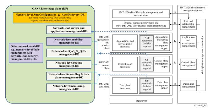
Figure I.3 – Illustrating the types of GANA DEs that can provide for autonomic decision support in applications and service plane management, control plane management and data plane management
