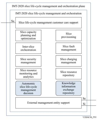
Figure 1 – High-level AMC architecture for IMT-2020 network slice life-cycle management
