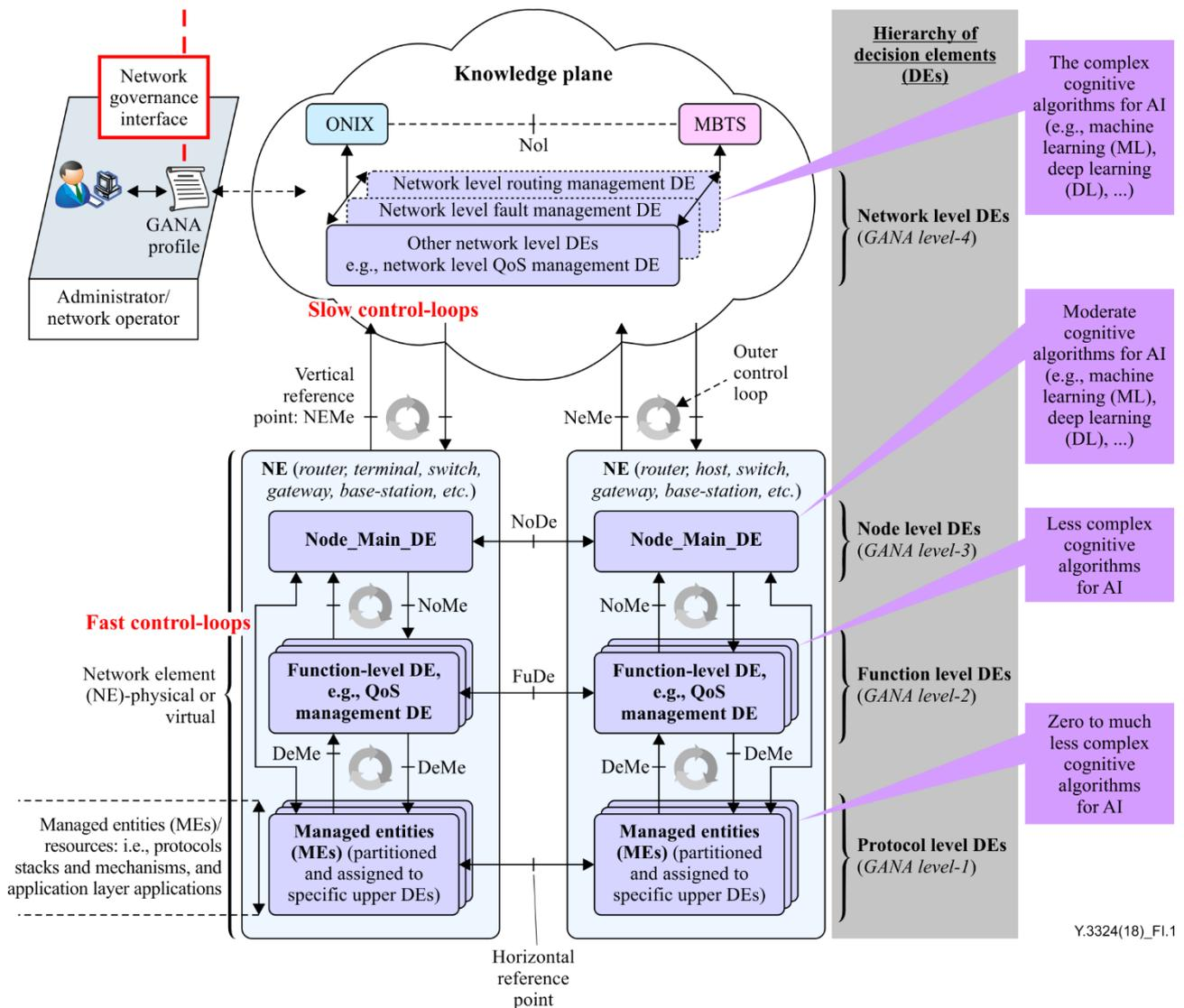
**Figure I.1 – Snapshot of the GANA reference model and autonomies cognitive algorithms for artificial intelligence (AI) (Source [b-ETSI PoC Demo-2])**
