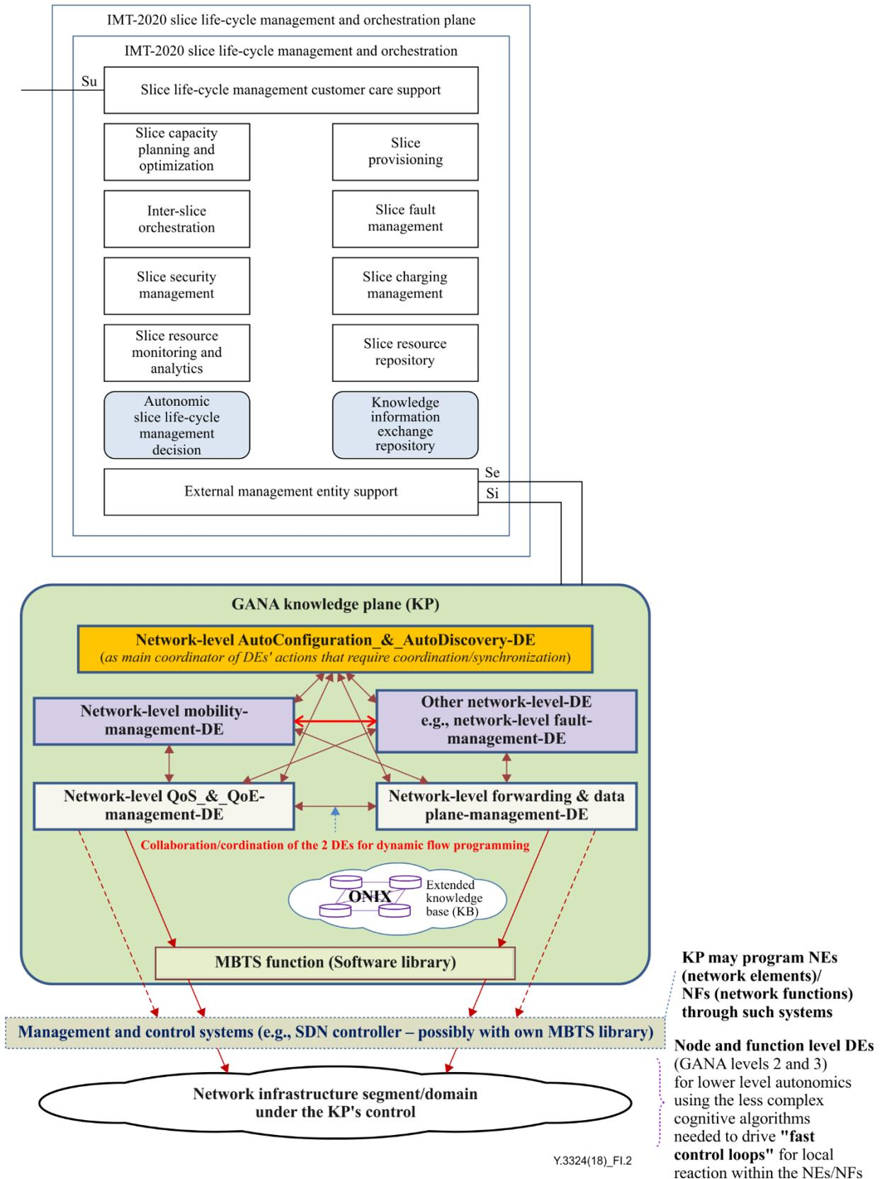
Figure I.2 – Illustration of how high-level AMC architecture for IMT-2020 network slice life-cycle management can be integrated with GANA functional blocks
