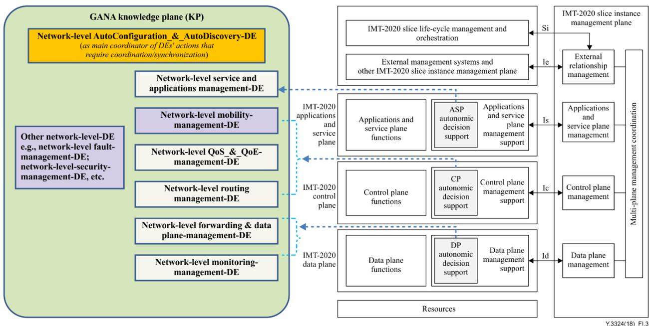
**Figure I.3 – Illustrating the types of GANA DEs that can provide for autonomic decision support in applications and service plane management, control plane management and data plane management**
