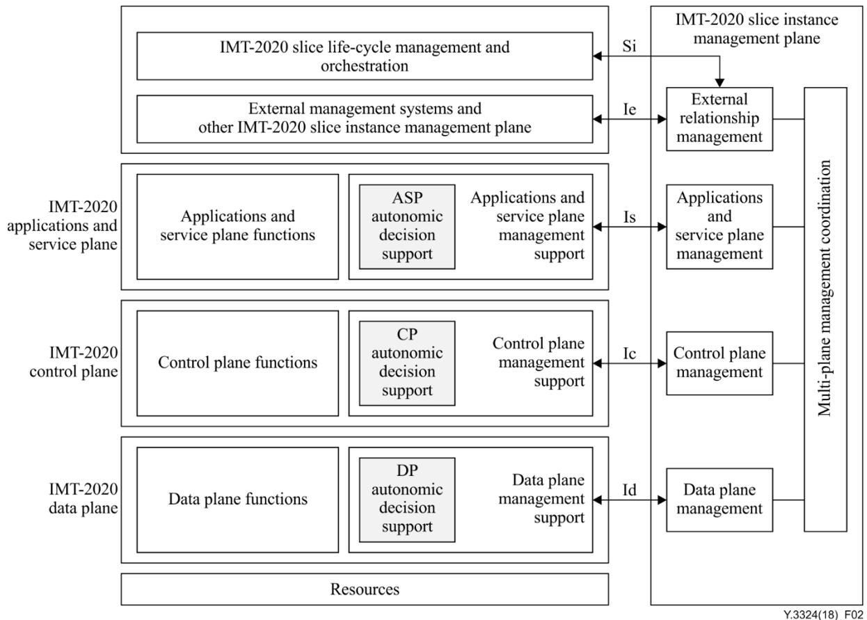
**Figure 2 – High-level AMC architecture for IMT-2020 network slice instance management**
