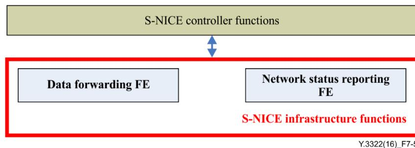
**Figure 7-5 – Detailed functional architecture of S-NICE infrastructure functions**
