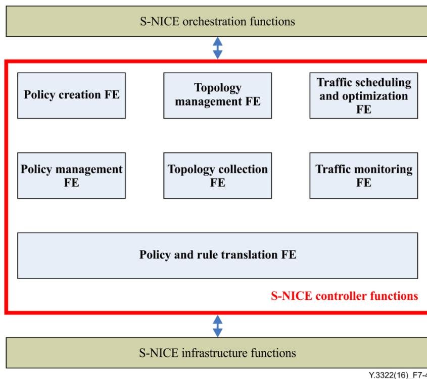
**Figure 7-4 – Detailed functional architectures of S-NICE controller functions**
