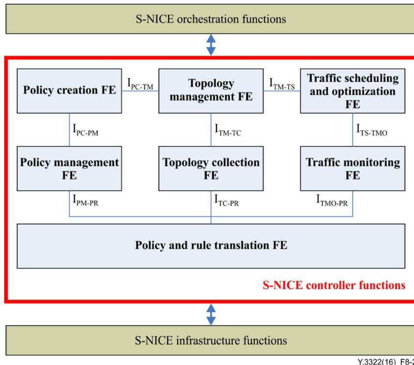
**Figure 8-2 – Internal reference points of S-NICE controller functions**
