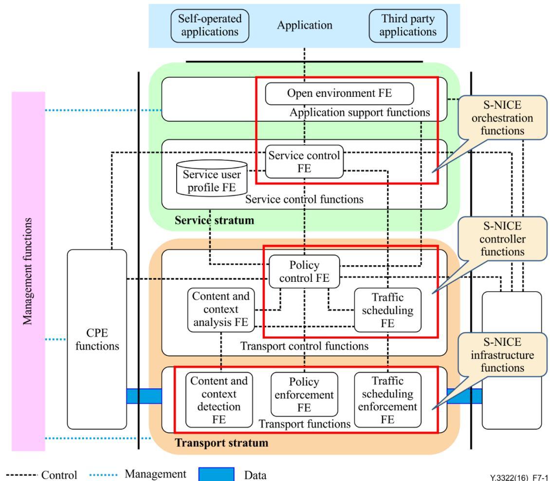
**Figure 7-1 – Relationship between architectures of NICE and S-NICE**
