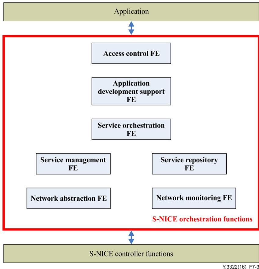
**Figure 7-3 – Detailed functional architectures of S-NICE orchestration functions**
