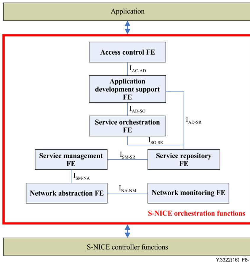
**Figure 8-1 – Internal reference points of S-NICE orchestration functions**
