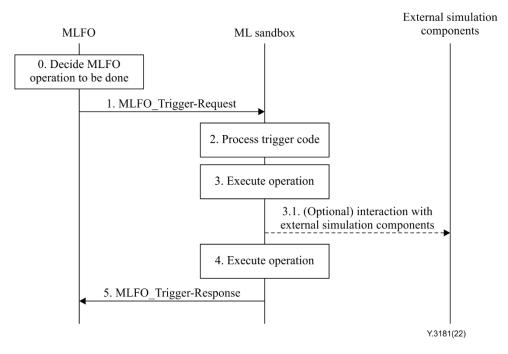
Figure 7 – MLFO-trigger operations
