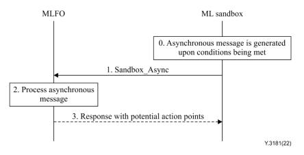
Figure 8 – ML sandbox asynchronous messages
