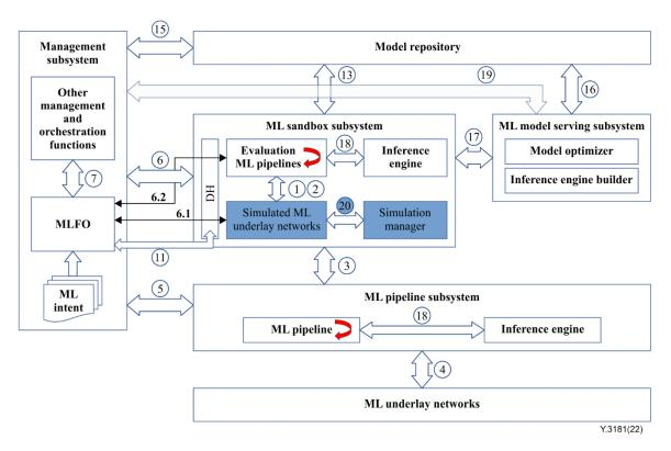
Figure 2 – ML sandbox within the high-level ML architecture
