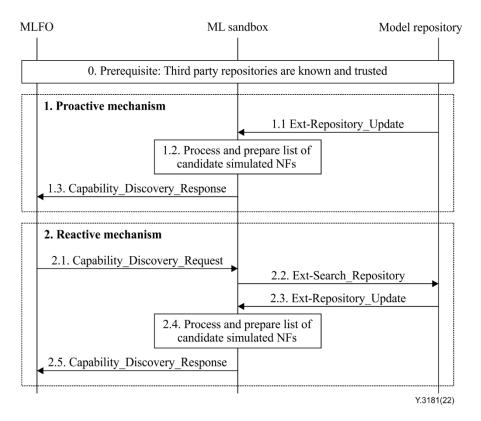
Figure 4 – Capability discovery for third-party simulation components
