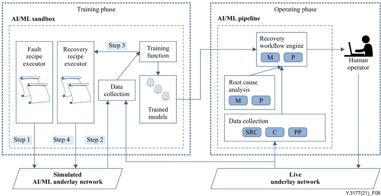
**Figure 8 – Functions and workflow of fault recovery with AI/ML**
