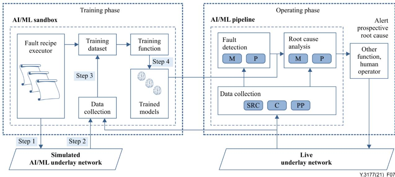
**Figure 7 – Functions and workflow of fault detection with AI/ML**
