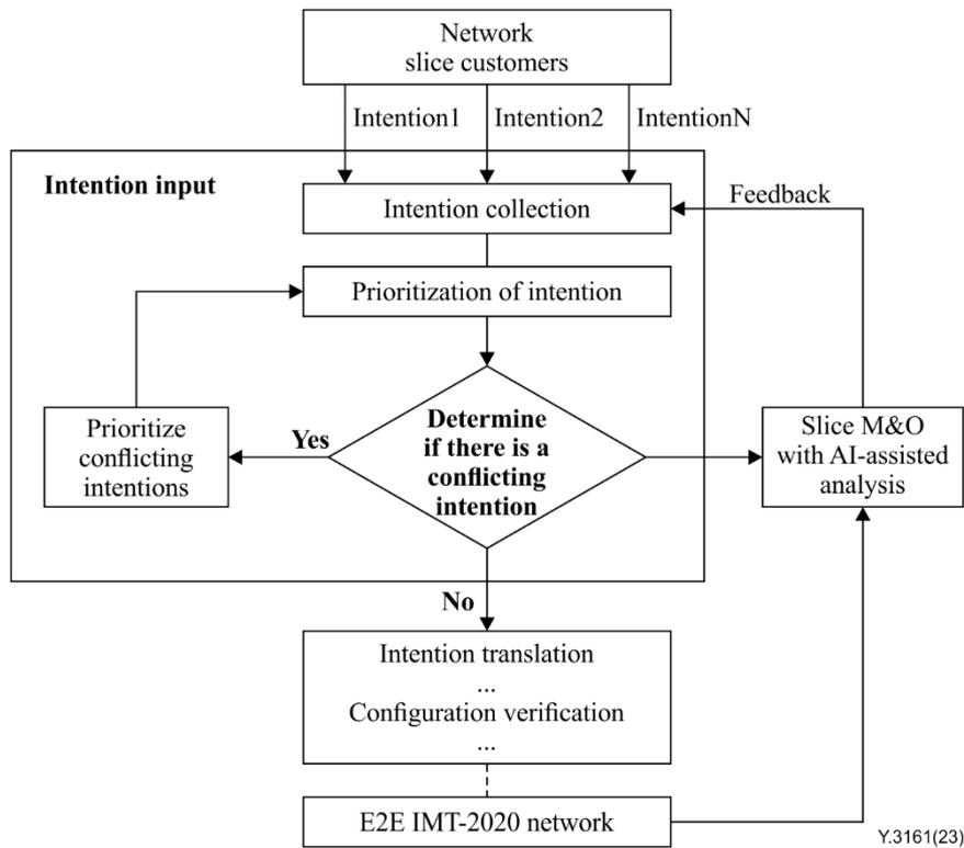
**Figure 9-1 – High-level method of multi-intention of network slice creation/modification**
