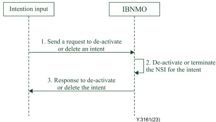
**Figure 10-6 – Procedure for de-activating or deleting an intent**
