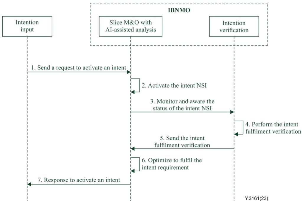
**Figure 10-3 – Procedure for activating an intent**
