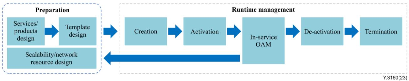
**Figure 8-1 – Network slicing lifecycle procedure [ITU-T Y.3154]**
