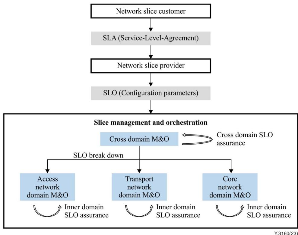
**Figure 6-1 – Overview of the architectural framework of end-to-end SLO guarantee**
