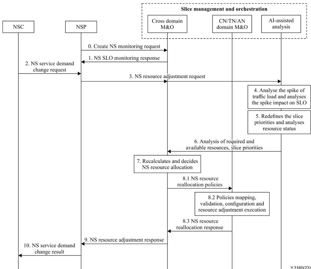
**Figure 8-3 – Procedures of NS resources adaptive adjustment**
