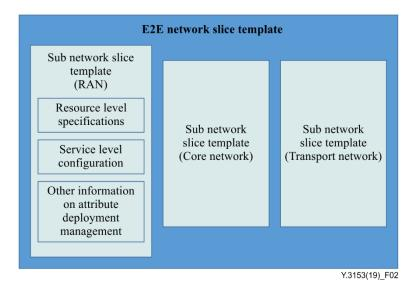
Figure 2 – Functional architecture of network slice template
