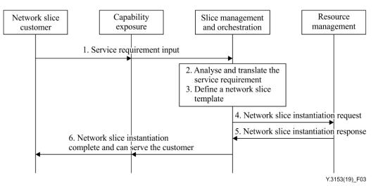
**Figure 3 – Procedure of network slice instantiation**
