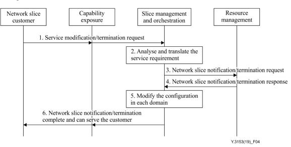
**Figure 4 – Procedure of network slice modification/termination**
