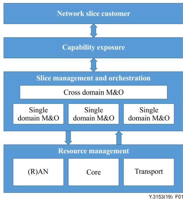
**Figure 1 – Functional architecture of network slice management and orchestration**
