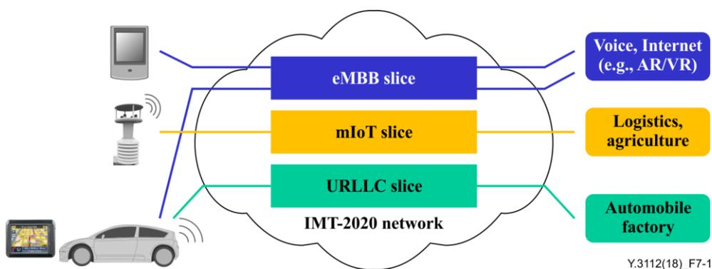
**Figure 7-1 – Use case for network slicing; Autonomous driving car**
