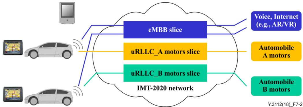
**Figure 7-2 – Use case where network slices are used to identify autonomous driving cars with different types of motor**
