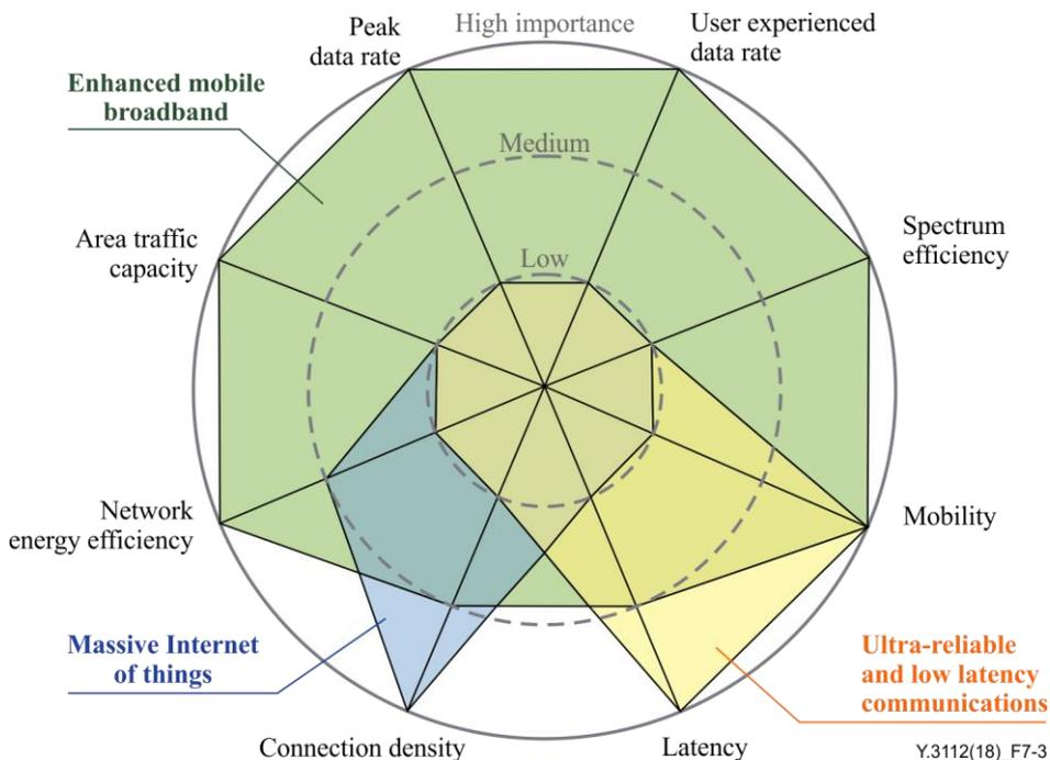
**Figure 7-3 – The importance of key capabilities in different usage scenarios**
