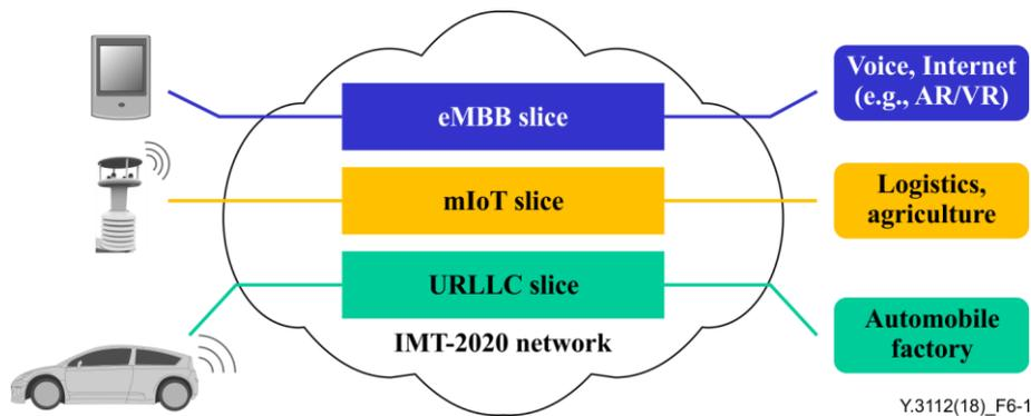
**Figure 6-1 – The concept of network slicing**
