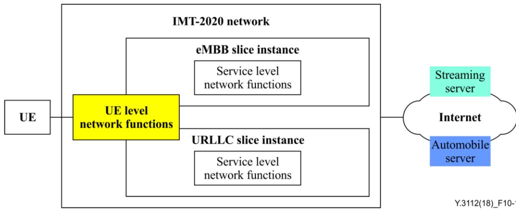
**Figure 10-1 – Network functions from the UE perspective**
