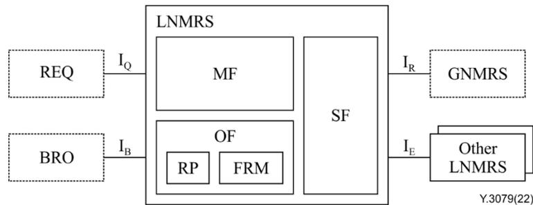
**Figure 3 – The architectural framework of locally enhanced name mapping and resolution**
