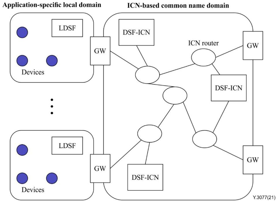
**Figure 1 – Components of ICN-based device registration and discovery framework**
