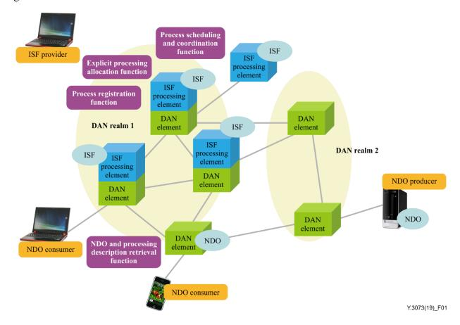
Figure 1 – Architecture for ICN service function chaining
