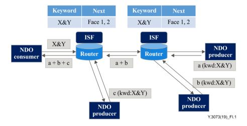
Figure I.1 – ISF forwarding requests and aggregating data
