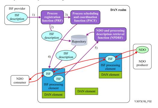
Figure 2 – Service function chaining mechanism
