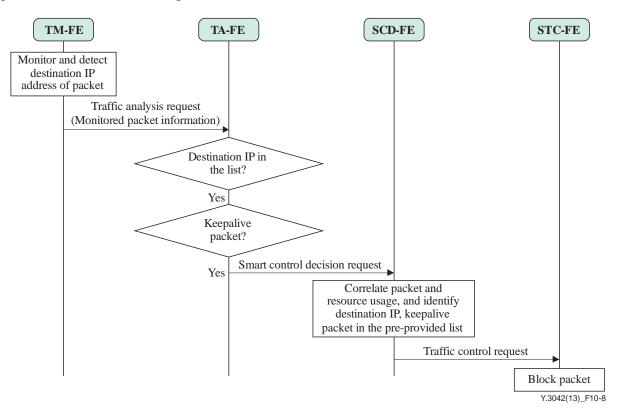
Figure 10-8 – Procedures for list-based traffic in P2P CDN
