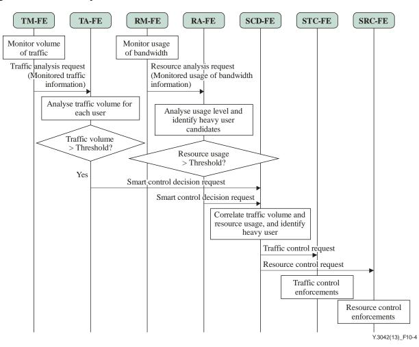
Figure 10-4 – Procedures of the heavy user traffic control mechanism
