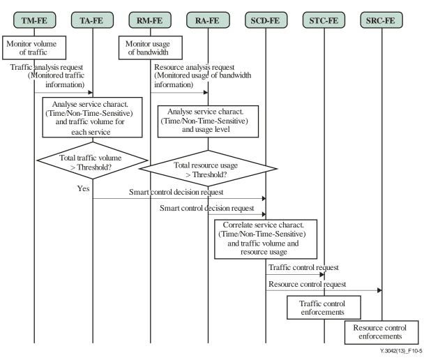
**Figure 10-5 – Procedures of the surge traffic control mechanism**
