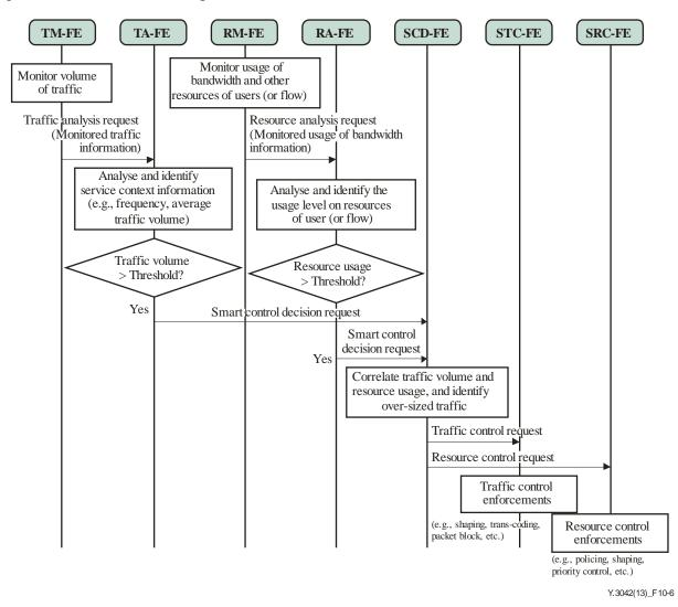
Figure 10-6 – Procedures for over-sized traffic
