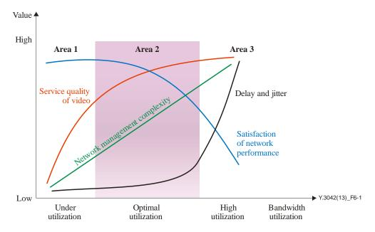
Figure 6-1 – Three different areas of network operation
