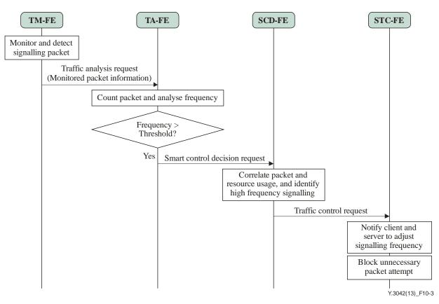
Figure 10-3 – Procedures for heavy signalling traffic
