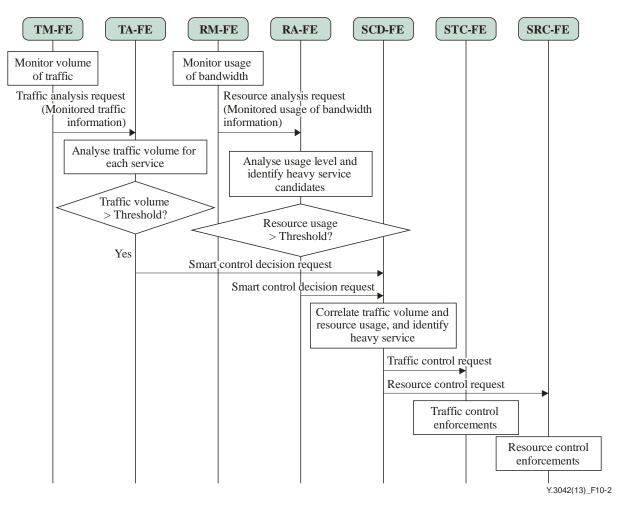
Figure 10-2 – Procedures for the heavy service traffic control mechanism
