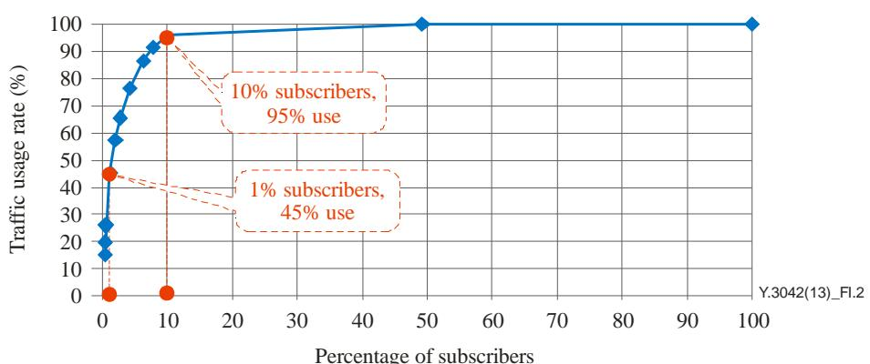
**Figure I.2 – Monopolization of traffic in mobile networks, 2010**
