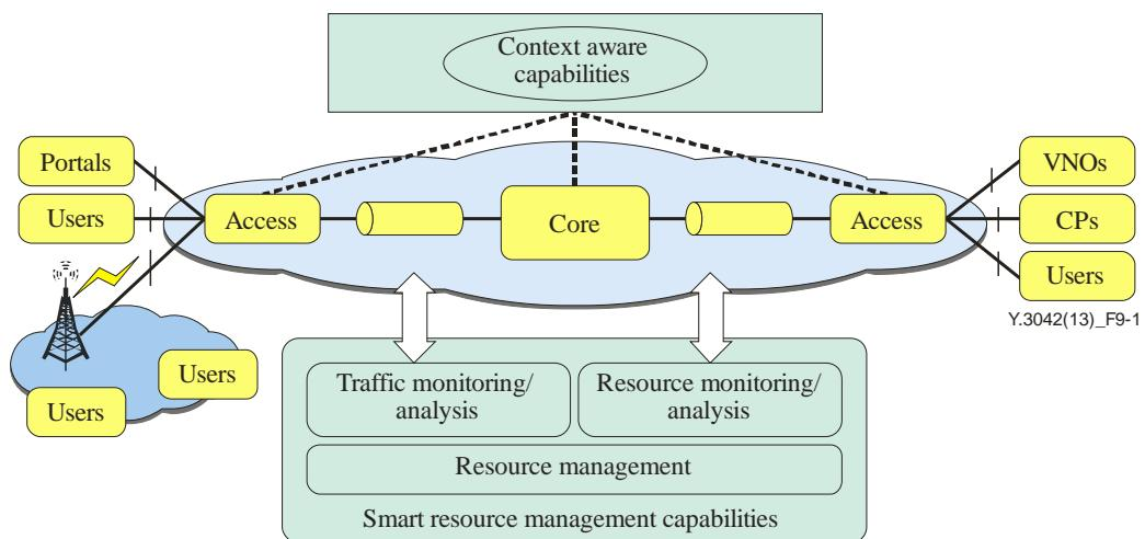
**Figure 9-1 – High level architecture of STCRMF**
