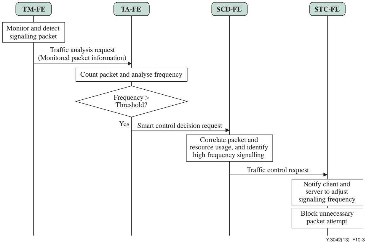
**Figure 10-3 – Procedures for heavy signalling traffic**
