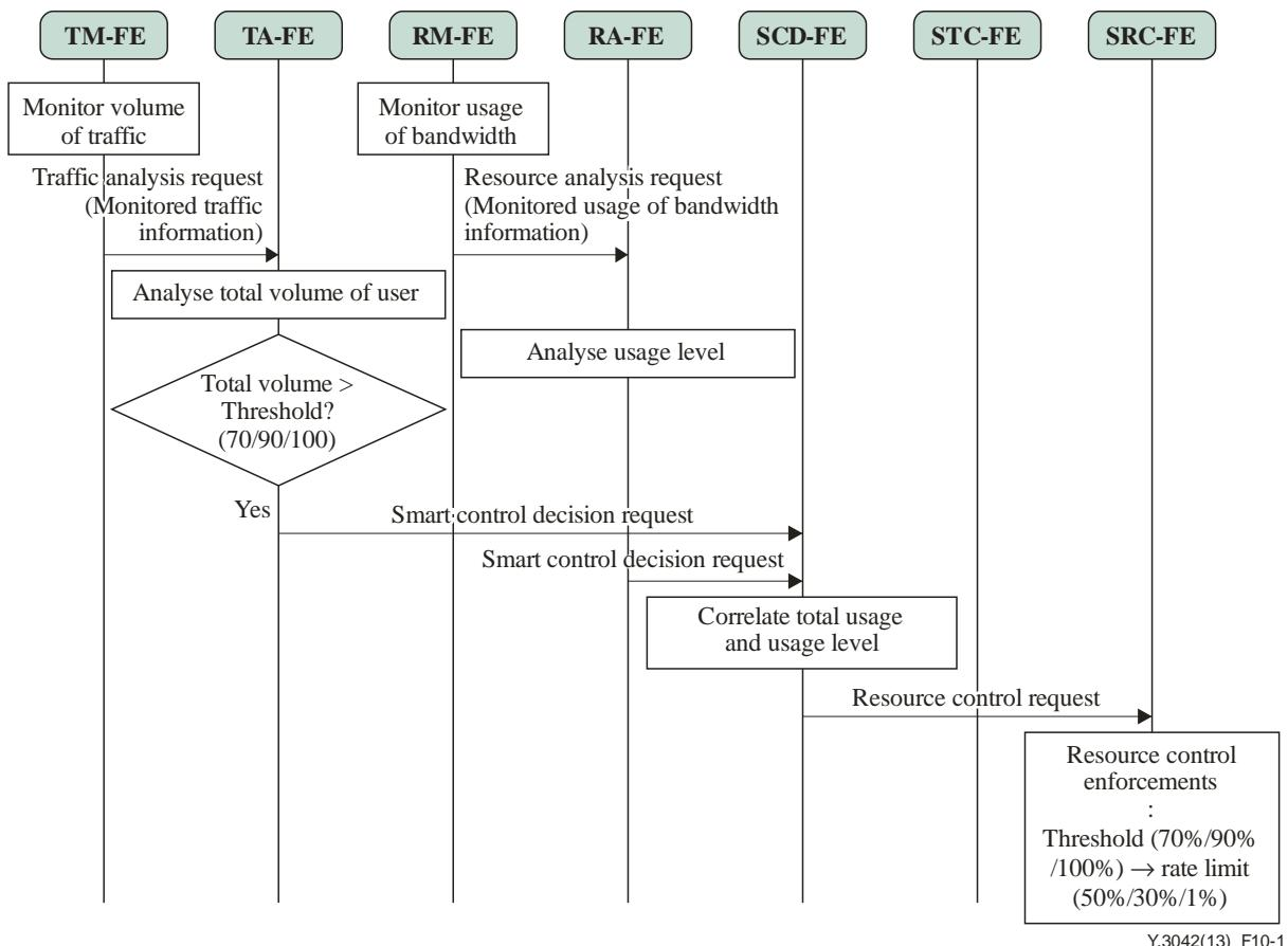
**Figure 10-1 – Procedures for the data cap based mechanism**
