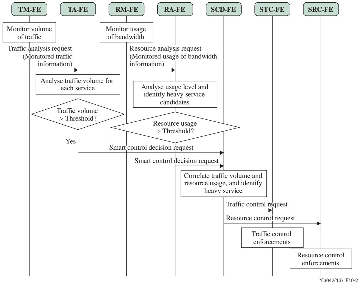
**Figure 10-2 – Procedures for the heavy service traffic control mechanism**
