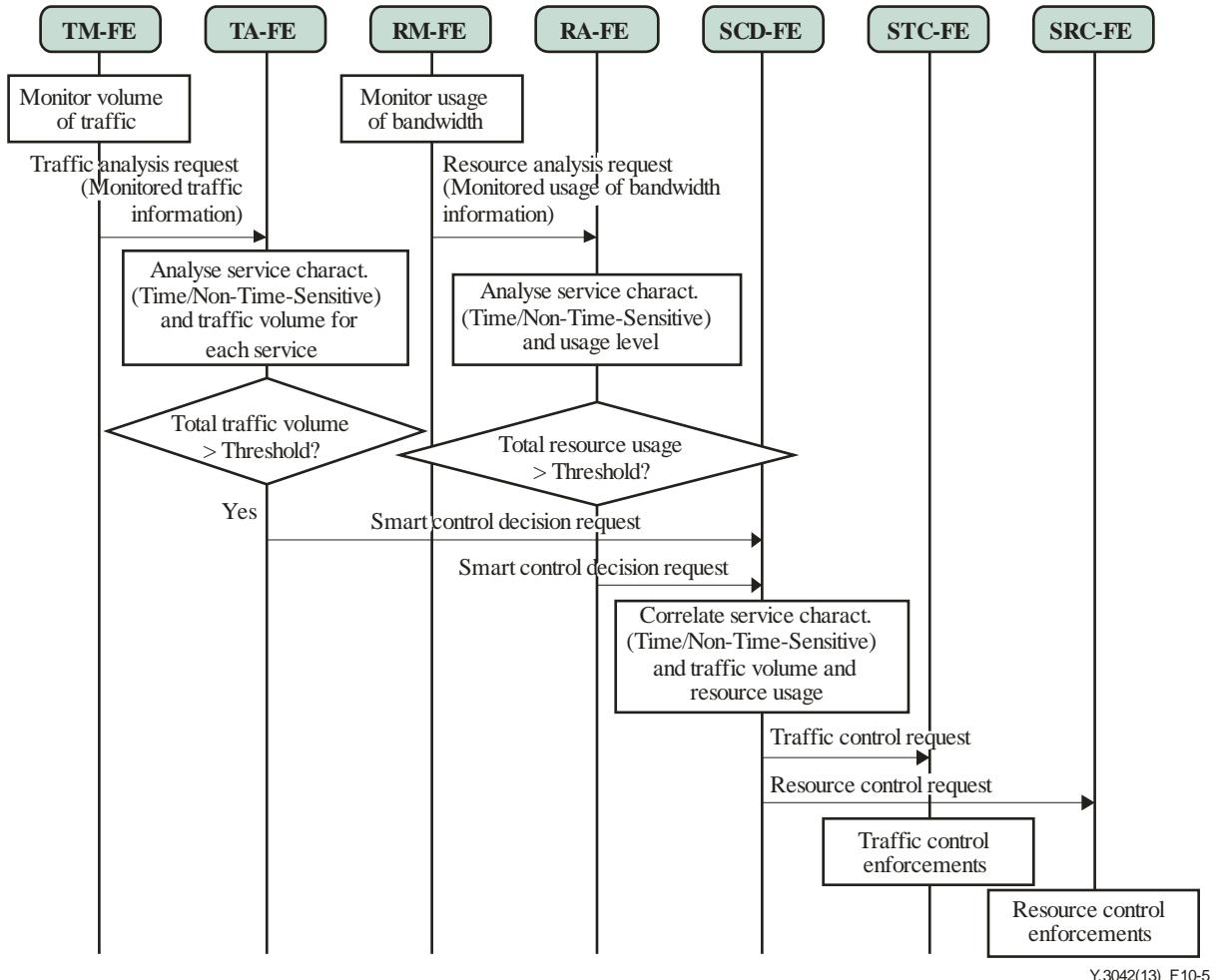
**Figure 10-5 – Procedures of the surge traffic control mechanism**
