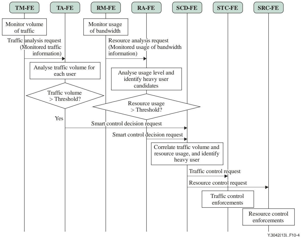
**Figure 10-4 – Procedures of the heavy user traffic control mechanism**
