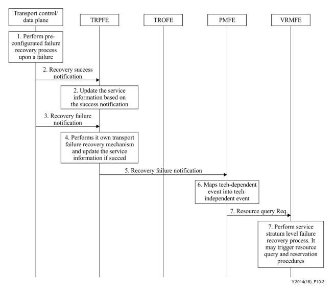
Figure 10-3 – Transport resource failure recovery procedure
