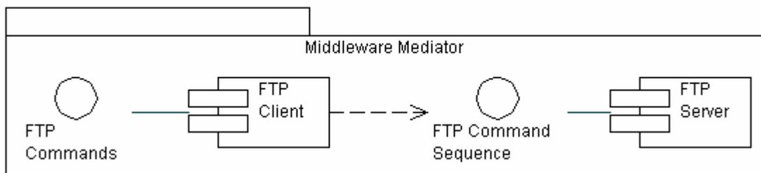
Figure C.2 - FTP Client-Server-Architecture
