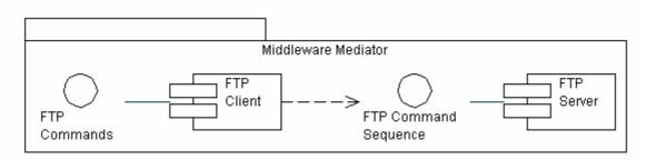
Figure C.2 - FTP Client-Server-Architecture
