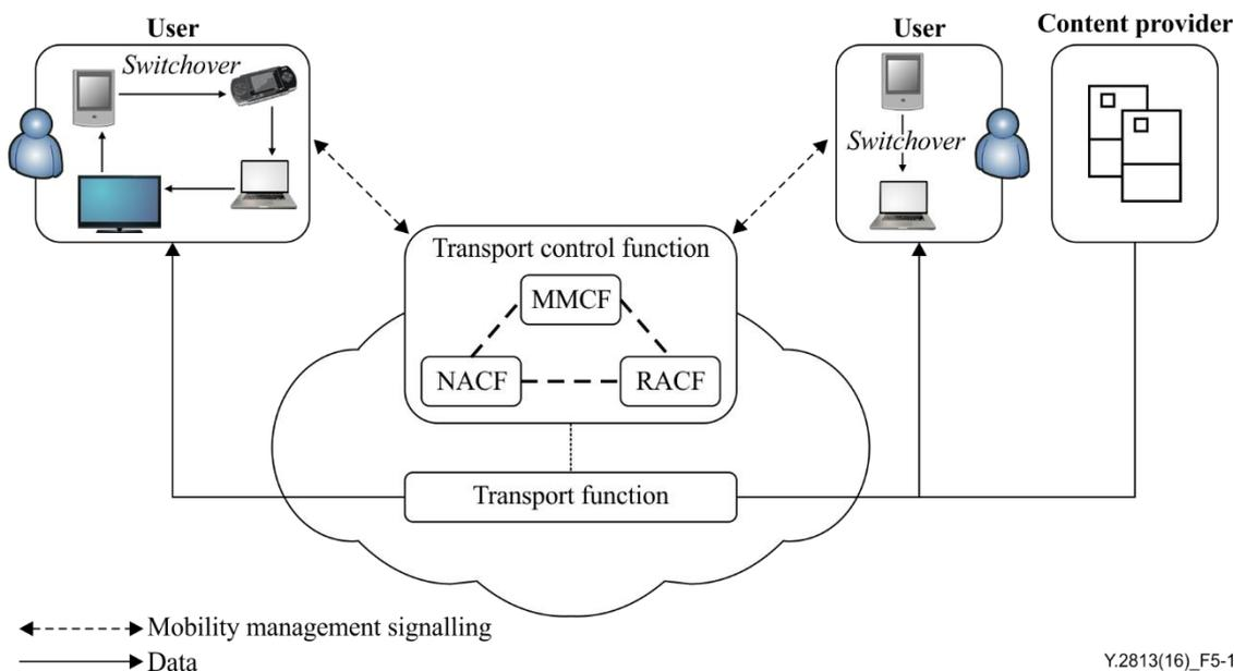
**Figure 5-1 – Mobility management for application using multiple devices**
