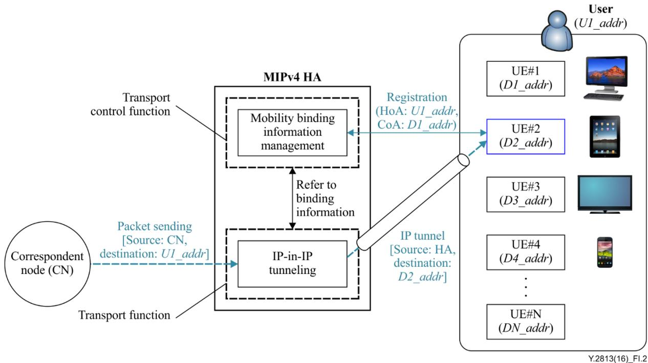
**Figure I.2 – Deployment of applications using MIPv4 (in case of one-to-multiple devices)**
