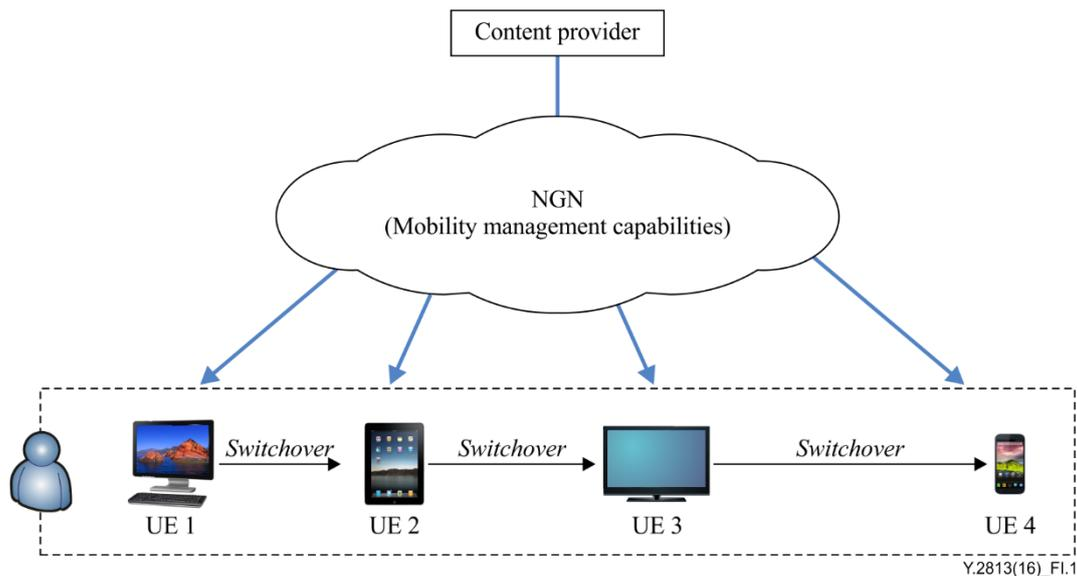
**Figure I.1 – Example of application with one-to-multiple devices**
