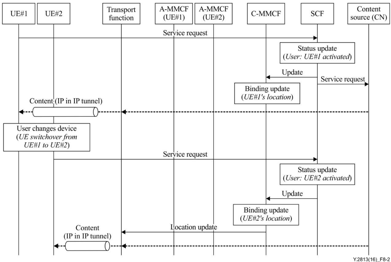
**Figure 8-2 – Procedure for application with one-to-multiple devices**
