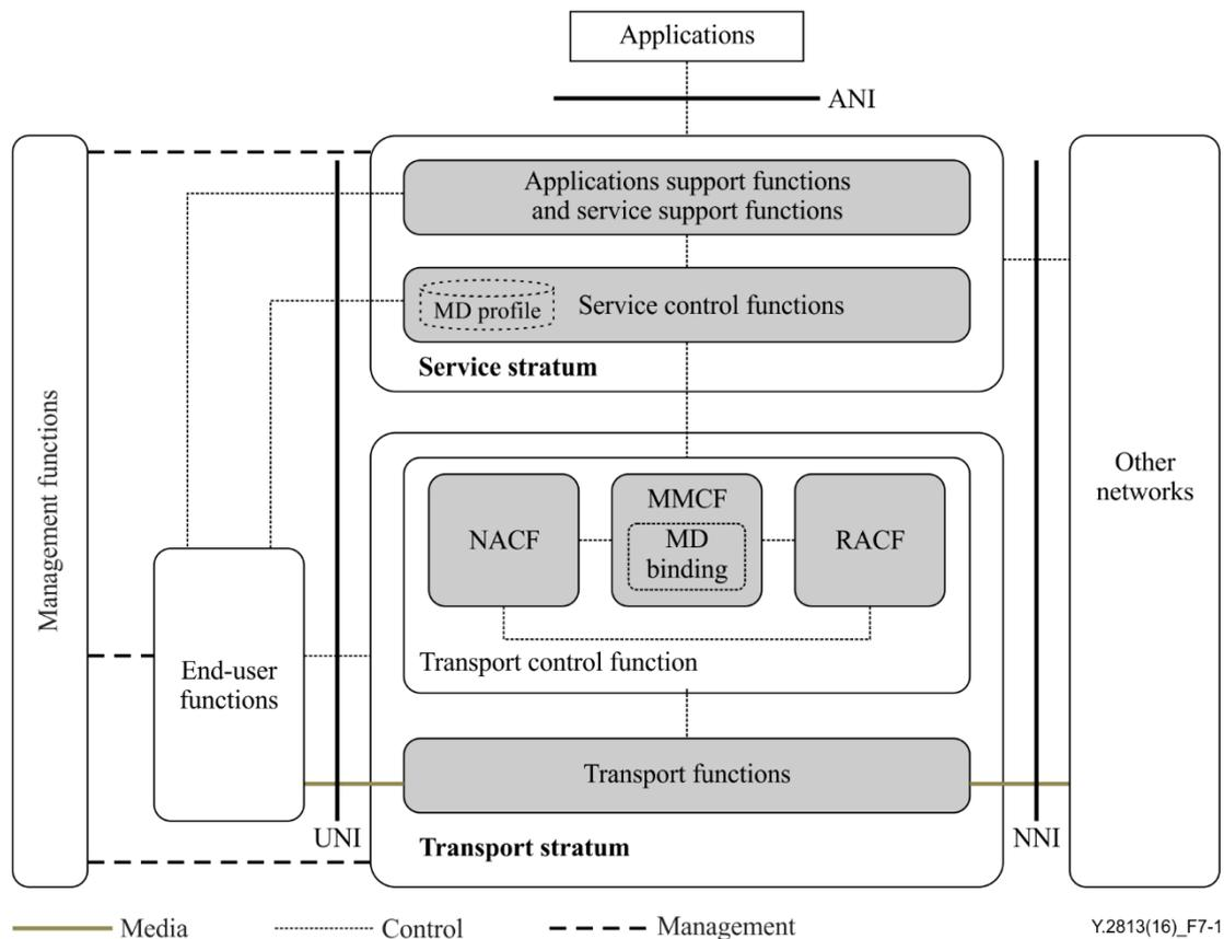
**Figure 7-1 – High level architecture for application with multiple devices based on [b-ITU-T Y.2012]**
