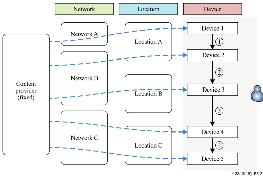
**Figure 5-2 – Scenario model of application with one-to-multiple devices (Case I)**
