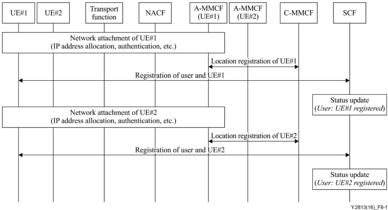
**Figure 8-1 – Procedure for registration of user and devices**
