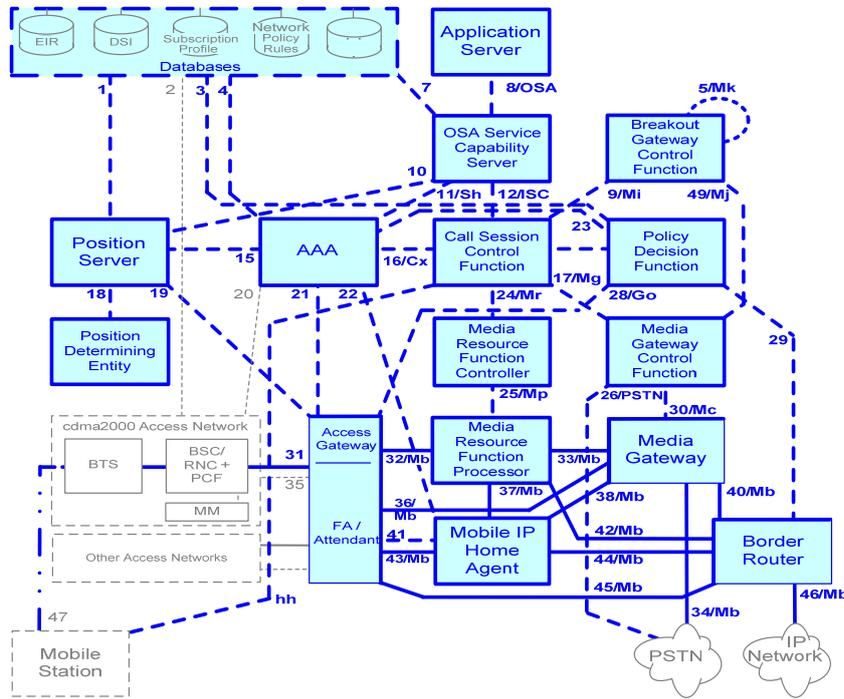
Figure I.3 – MMD network architecture model
