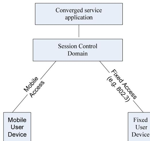
**Figure 7 – FMC between IMS controlled packet switched networks**
