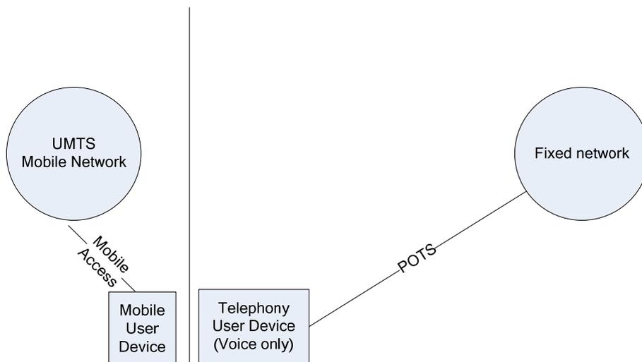
**Figure 6 – Service continuity between telephony terminals**
