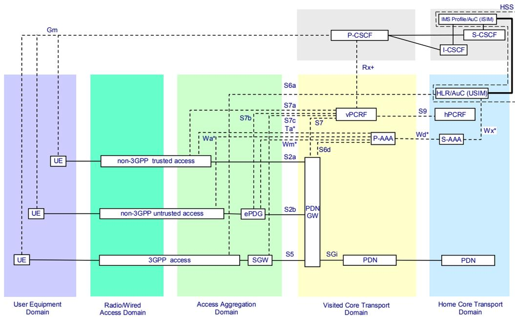
**Figure I.7 – Mapping of local break-out architecture to IMS-based FMC reference model**
