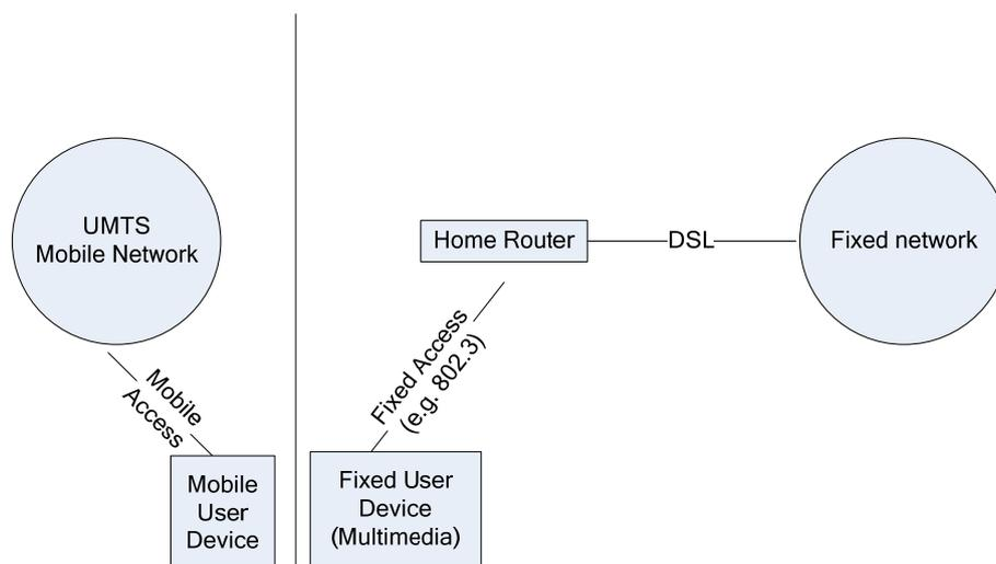
**Figure 5 – Service continuity between different multimedia terminals**
