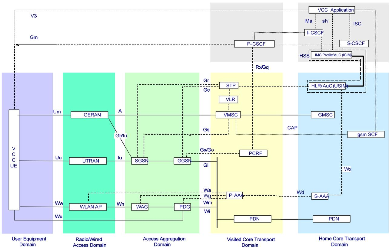
**Figure I.8 – Mapping of 3GPP VCC architecture to IMS-based FMC reference model**
