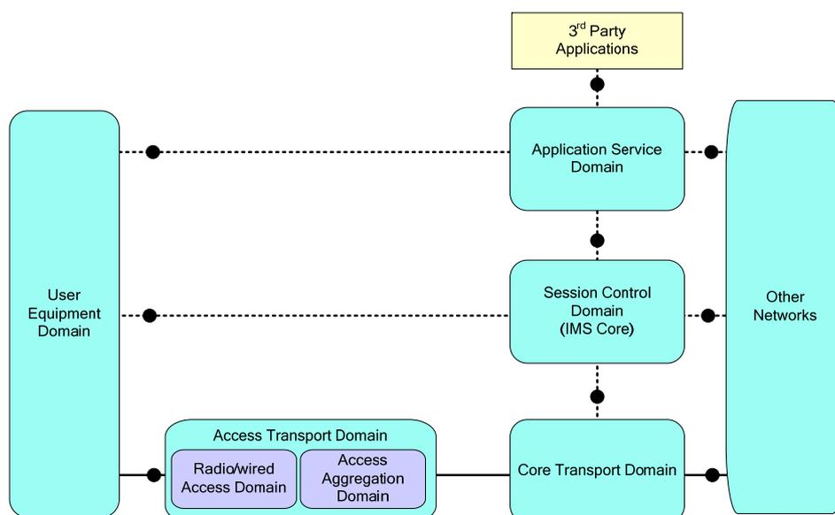
**Figure 2 – IMS based NGN reference model**
