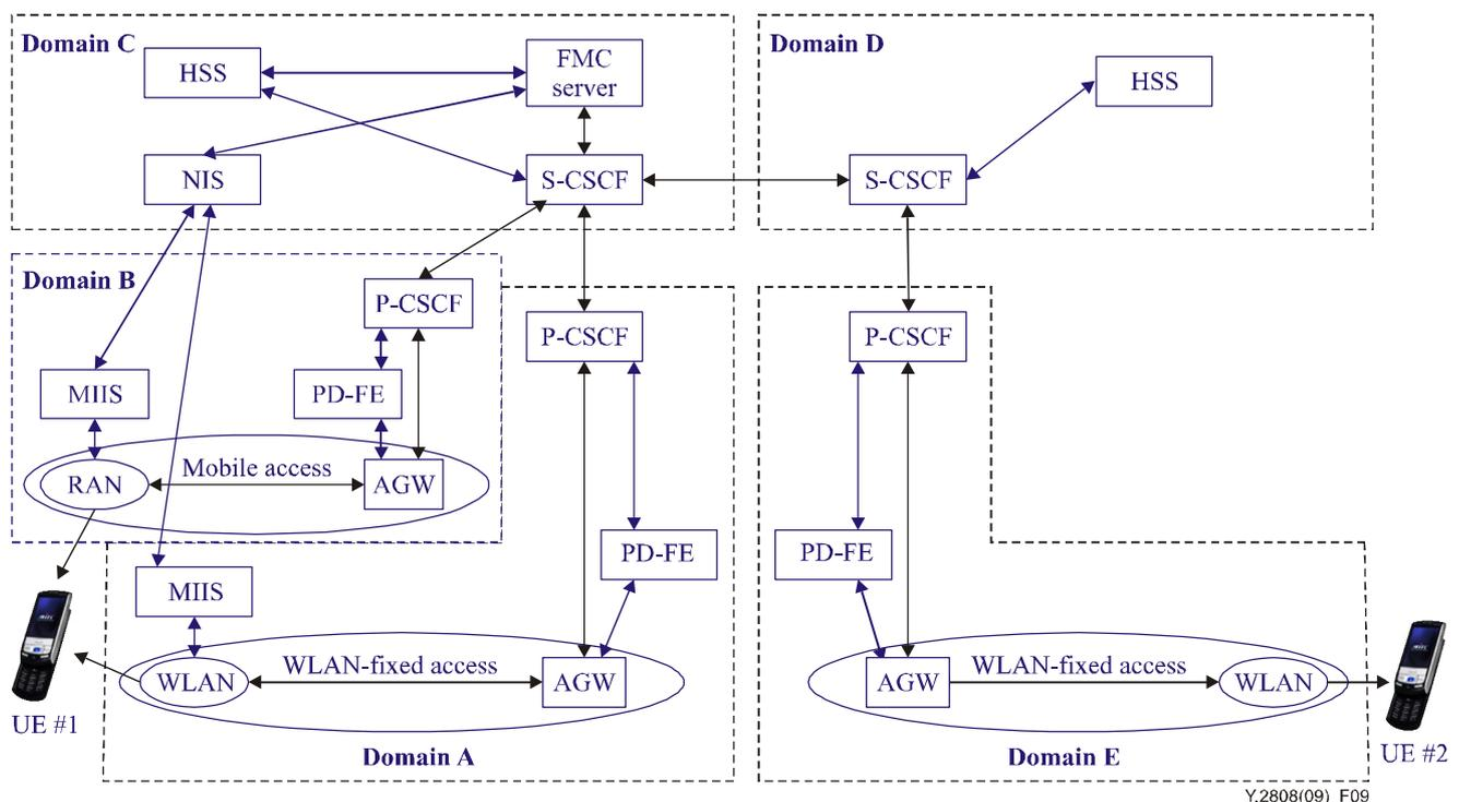
**Figure 9 – PS-PS service level convergence architecture**
