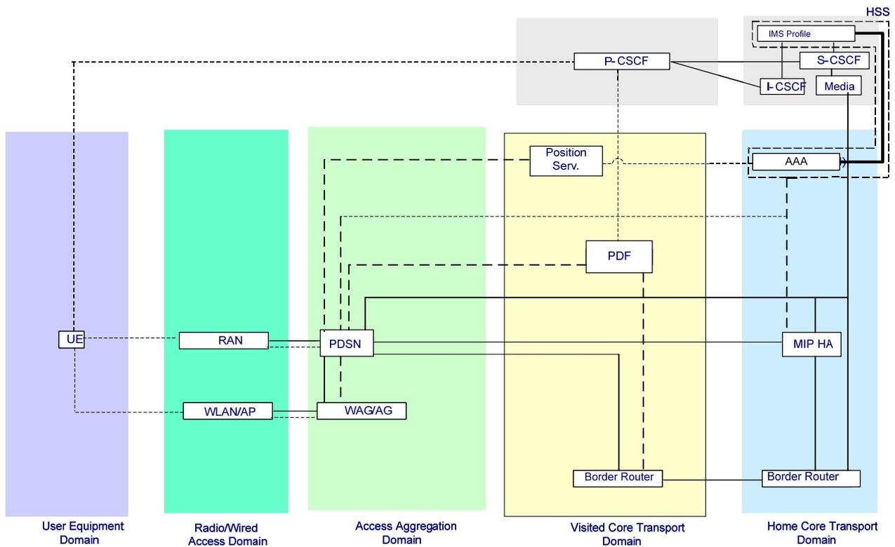
**Figure I.4 – Mapping of 3GPP2 architecture (with home routed traffic) to IMS-based FMC reference model**
