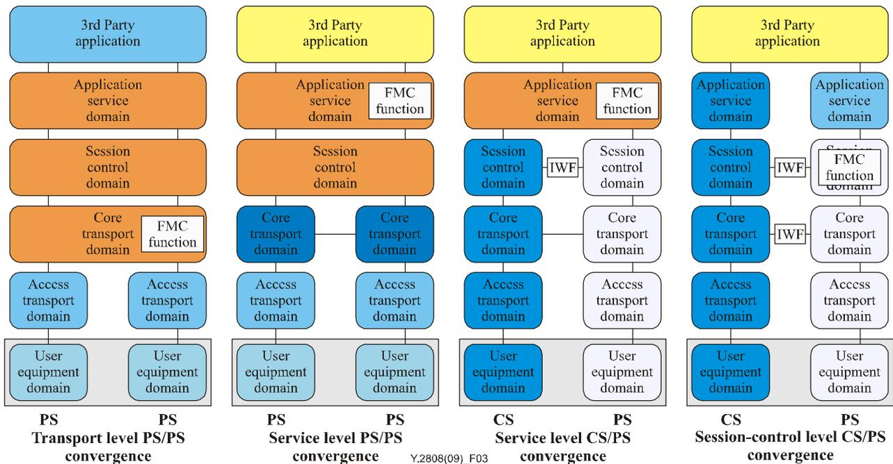
**Figure 3 – Convergence point and FMC function**
