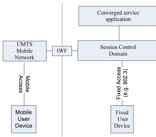
**Figure 8 – FMC between an IMS controlled packet switched network and CS mobile networks**
