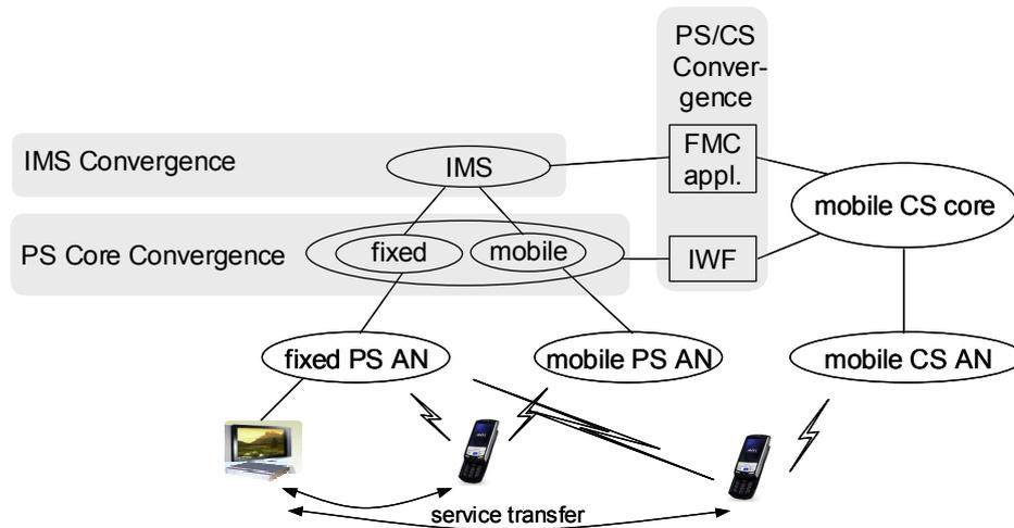
**Figure 1 – High-level IMS based FMC architecture**
