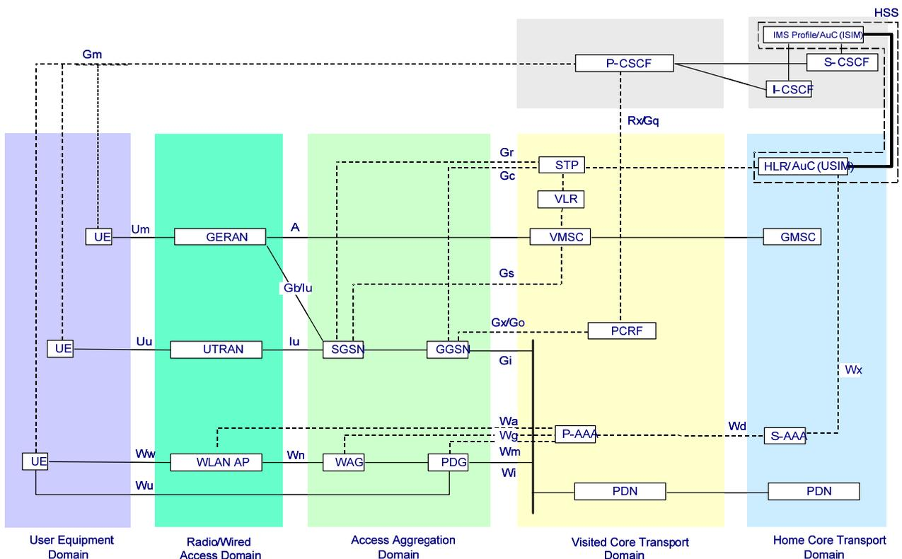
**Figure I.2 – Mapping of 3GPP architecture to IMS-based FMC reference model**
