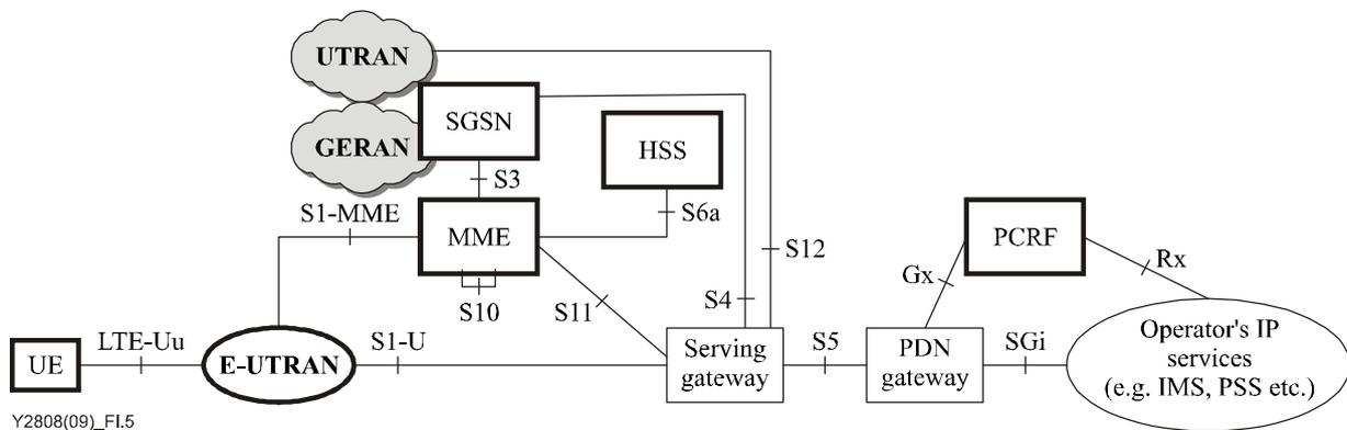
**Figure I.5 – Non-roaming architecture for 3GPP accesses**
