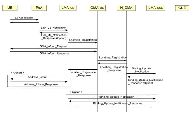
Figure II.4 – Information flow for location update in case UE is located in a foreign core network, and CUE in the home core network
