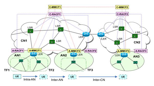
Figure 8-1 – Mobility scenarios across access networks connected to MPLS-based NGN core networks
