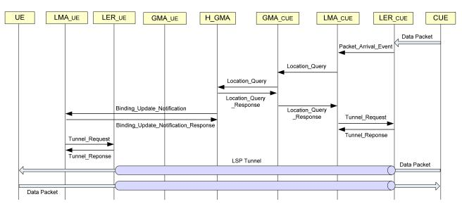
Figure II.8 – Information flow for location query/response in case UE and CUE are located within different foreign core networks
