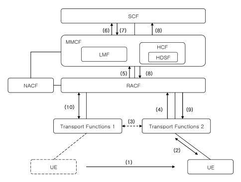
Figure I.4 – Handover functional procedure in the case of downgraded service
