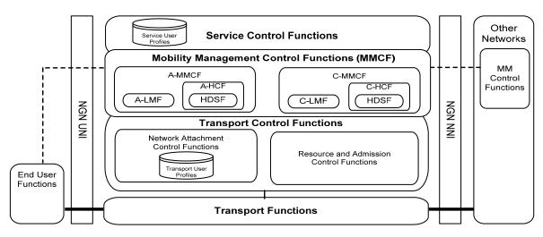
Figure 7-2 – Functional architecture for support of MPLS-based mobility capabilities
