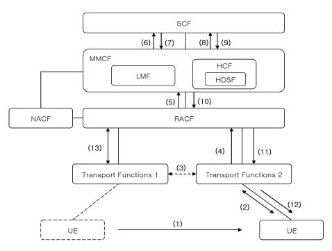
Figure I.5 – Handover functional procedure in the case of no resources
