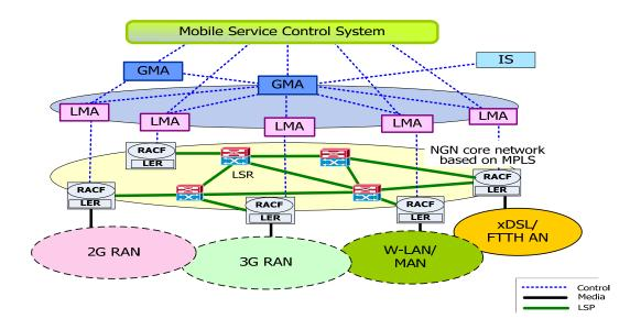
Figure 7-1 – Network environment with support of MPLS-based mobility capabilities
