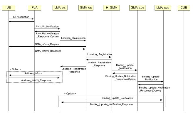
Figure II.5 – Information flow for location update in case UE and CUE are located in a foreign core network
