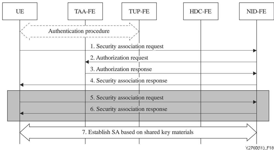
**Figure 18 – Security association establishment procedure based on PKI**
