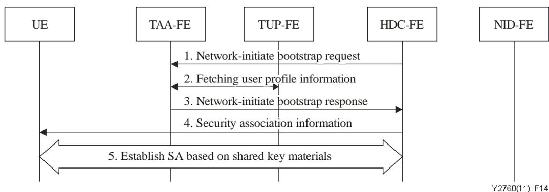
**Figure 14 – Network-initiated security association establishment procedure**
