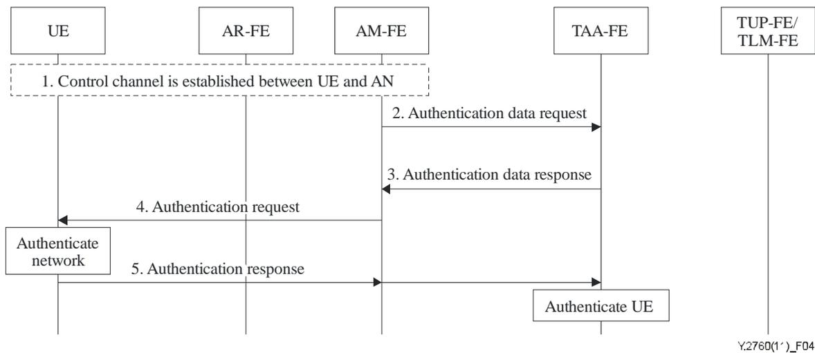
**Figure 4 – Generic fast re-authentication procedure**
