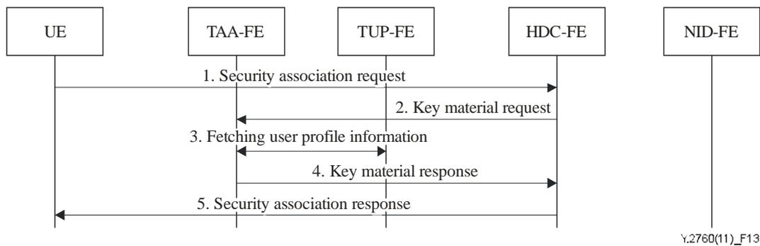
**Figure 13 – Host-initiated security association establishment procedure**
