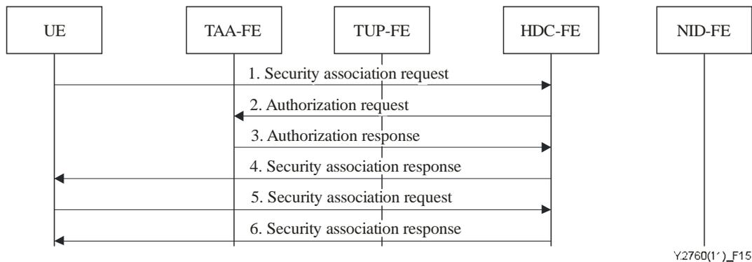
**Figure 15 – Security association establishment procedure based on PKI**
