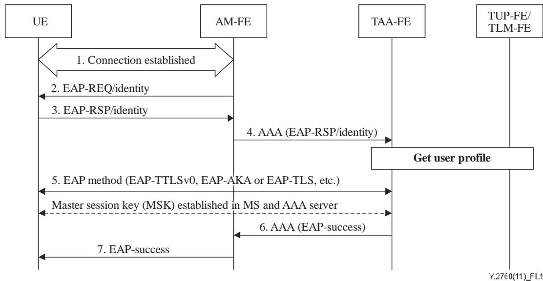
**Figure I.1 – Full authentication procedure**
