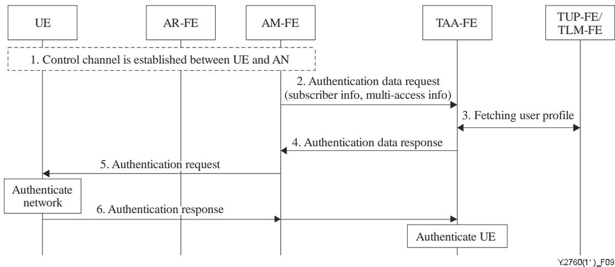
**Figure 9 – Multi-connection based authentication**
