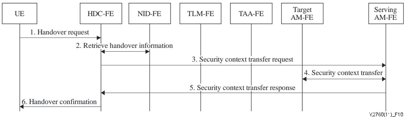
**Figure 10 – Host-initiated security context transfer procedure**
