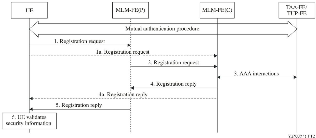
**Figure 12 – Host-based mobility procedure**
