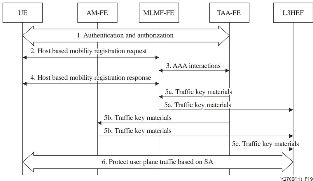
**Figure 19 – User plane traffic security between UE and L3HEF procedure**
