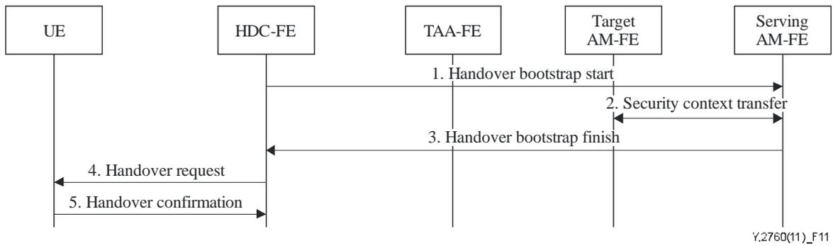
**Figure 11 – Network-initiated security context transfer procedure**
