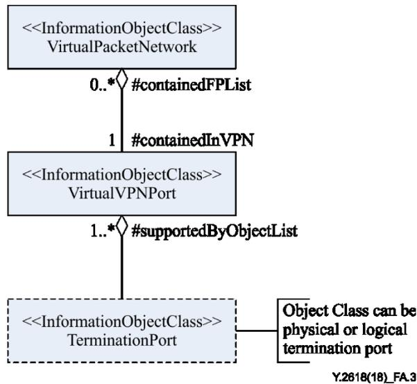
**Figure A.3 – ER diagram of virtual packet network fragment**
