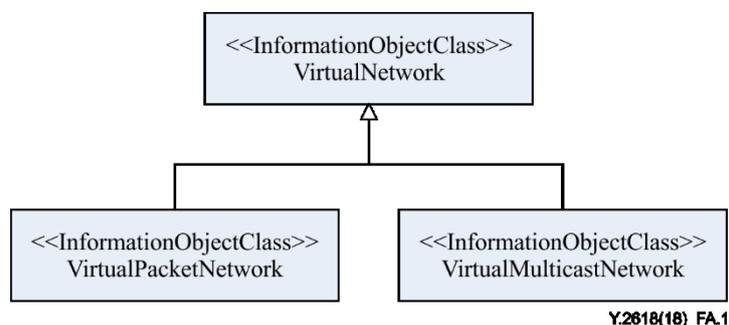
Figure A.1 – Inheritance diagram of virtual network fragment
