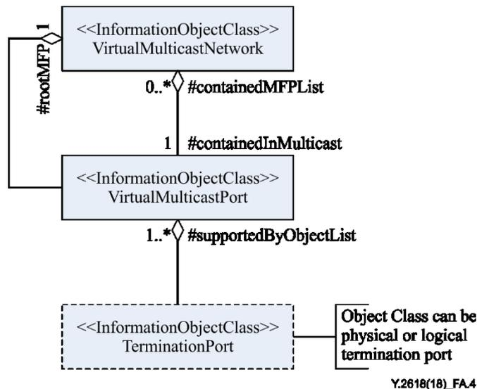
Figure A.4 – ER diagram of virtual multicast network fragment
