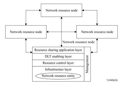
Figure 7-1 – General framework of network resource sharing based on distributed ledger technology
