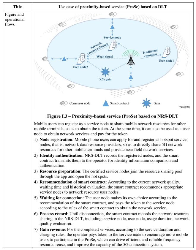
Table I.3 – Use case of proximity-based service (ProSe) based on NRS-DLT
