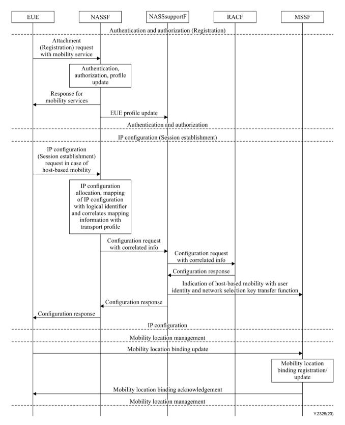
Figure I.1 – Information flows for attachment, case of host-based mobility
