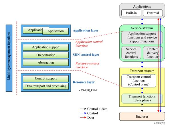
Figure 8-7 – Handling of built-in services in evolved NGN architecture based on SDN technology
