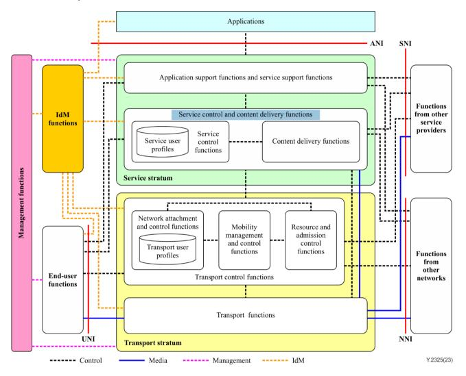
Figure 8-8 – Existing NGN architecture and high-level functions [Source: ITU-T Y.2012]
