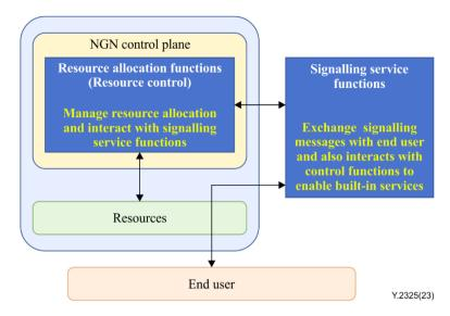
Figure 8-3 – Decoupled signalling service functions from the NGN control plane
