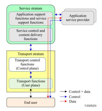
Figure 8-6 – Interfaces between an external application and NGN
