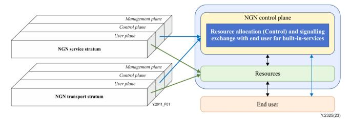
Figure 8-1 – Overview of the existing NGN architecture and high-level functionality distribution
