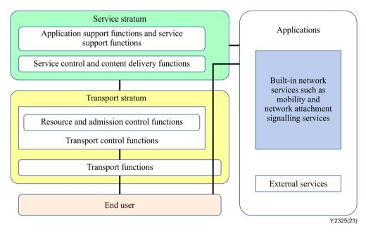
Figure 8-5 – Architecture overview for evolved NGN control plane
