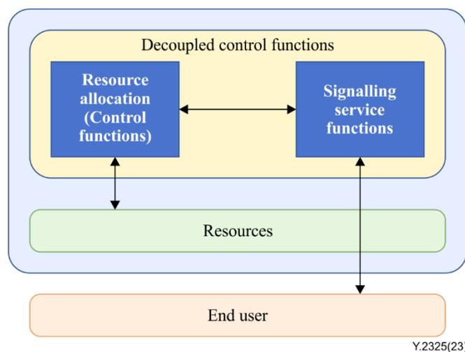
**Figure 8-2 – Decoupling of resource control functions and signalling handling functions in control plane**
