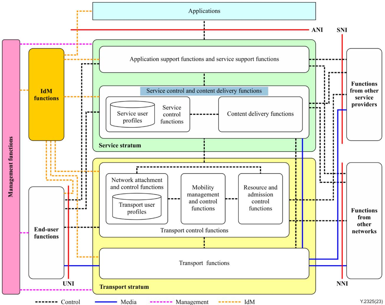
**Figure 8-8 – Existing NGN architecture and high-level functions**
