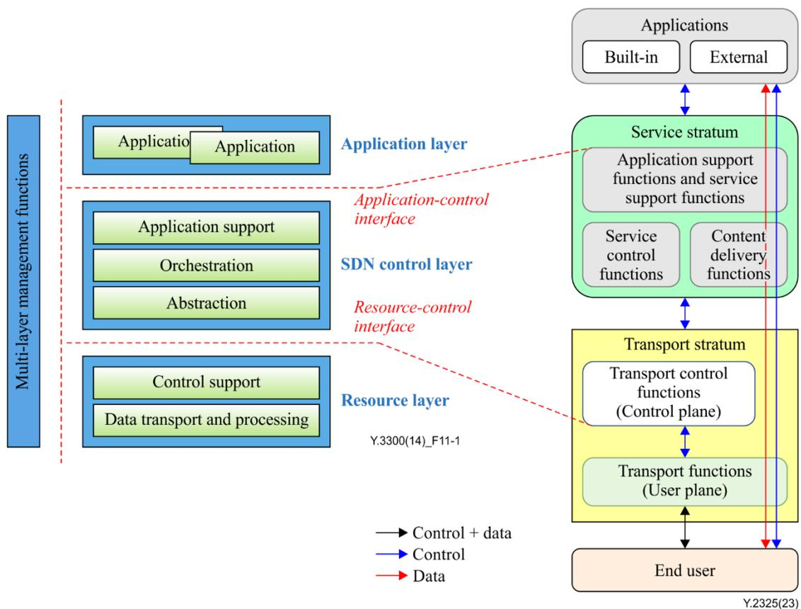
**Figure 8-7 – Handling of built-in services in evolved NGN architecture based on SDN technology**
