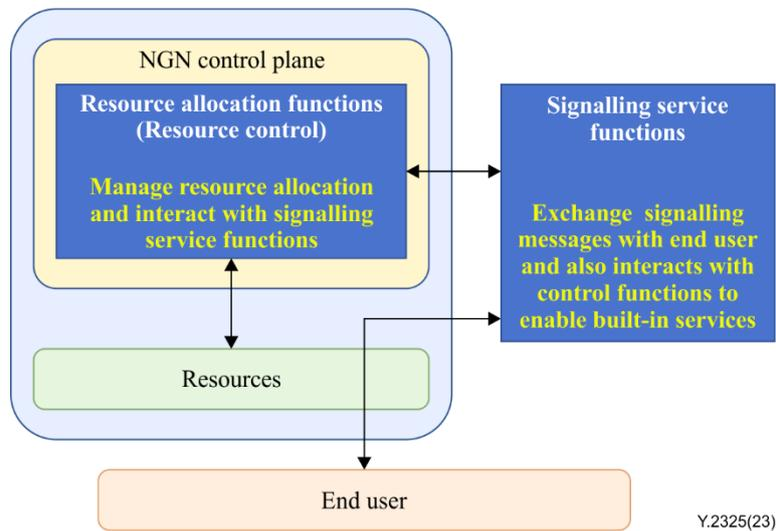
**Figure 8-3 – Decoupled signalling service functions from the NGN control plane**
