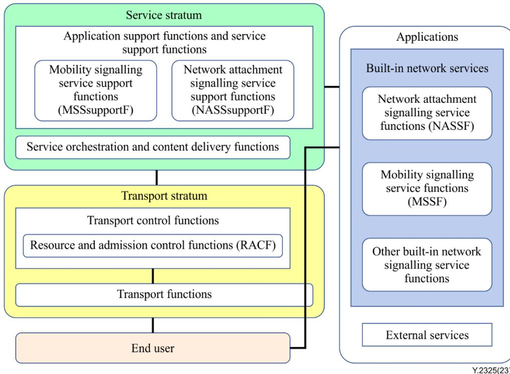
**Figure 8-9 – Placement and splitting of high-level functions for network attachment and mobility services in evolved NGN**
