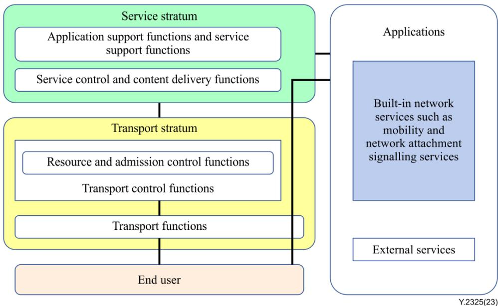
**Figure 8-5 – Architecture overview for evolved NGN control plane**
