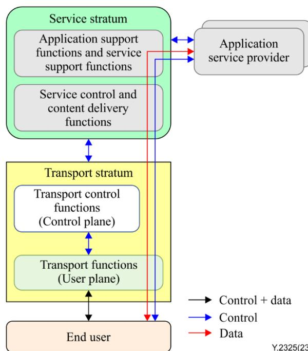
**Figure 8-6 – Interfaces between an external application and NGN**
