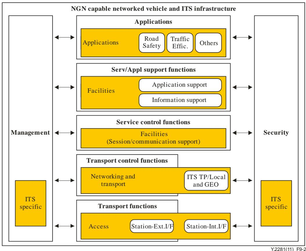
**Figure 9-2 – Reference architecture of NGN-capable networked vehicle and ITS infrastructure**
