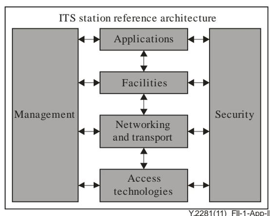
**Figure II.1 – ITS station reference architecture**
