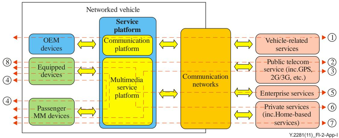
**Figure I.2 – Classification of use cases for communication of a networked vehicle**
