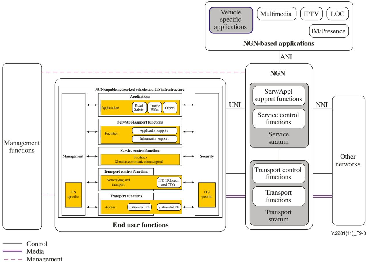
**Figure 9-3 – Overview architecture of NGN-capable networked vehicle and ITS infrastructure in cooperation with NGN**
