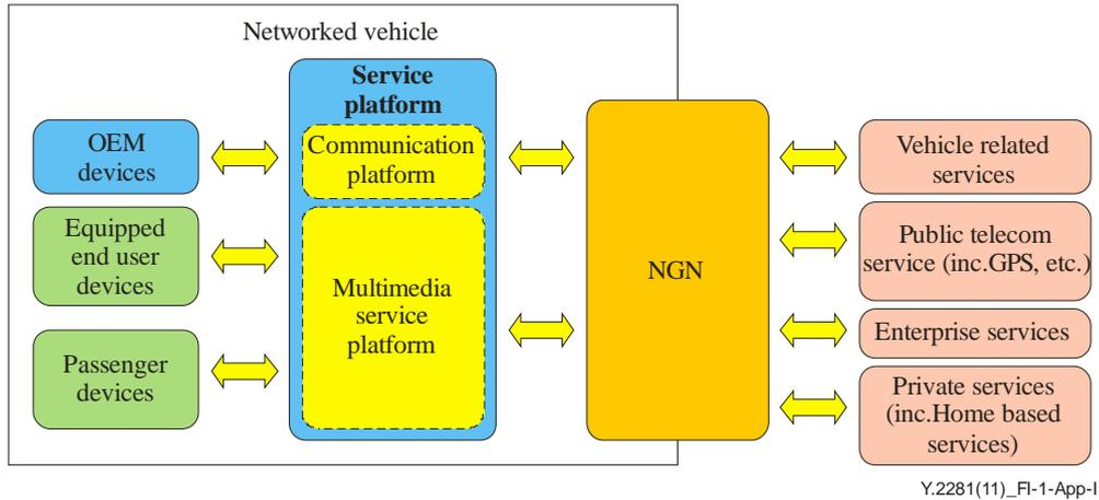
**Figure I.1 – Service configuration model of a networked vehicle**
