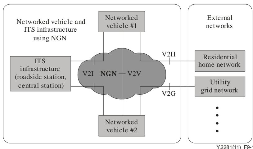
**Figure 9-1 – Overall configuration model of networked vehicle and ITS infrastructure**
