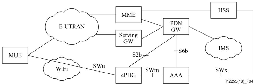
**Figure 4 – Network architecture with ePDG**
