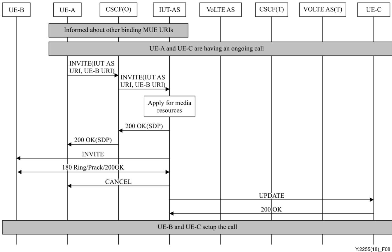
**Figure 8 – MUE transfer to other devices by switching to specified MUE**
