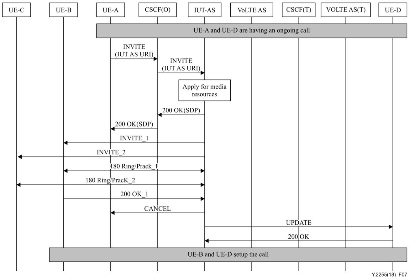
**Figure 7 – MUE transfer to other devices by notifying all binding terminals**
