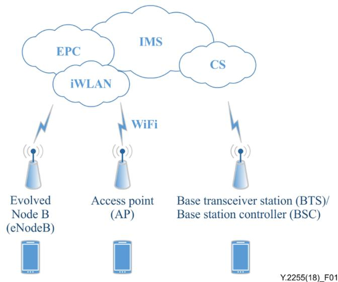
**Figure 1 – The architecture for VCC over multi-connection**
