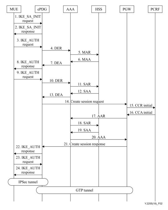
Figure 2 – Initial attachment via Wi-Fi access
