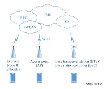
Figure 1 – The architecture for VCC over multi-connection
