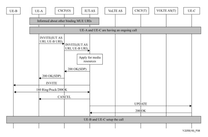
Figure 8 – MUE transfer to other devices by switching to specified MUE
