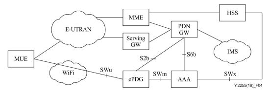
Figure 4 – Network architecture with ePDG
