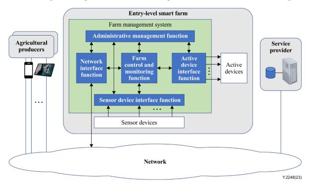
Figure 2 – Reference architecture for entry-level smart farm
