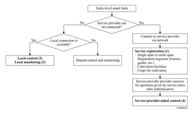
Figure 3 – Relation between infrastructure condition and service features in entry-level smart farms
