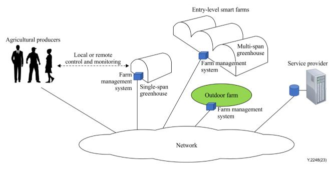
Figure 1 – Conceptual diagram of entry-level smart farm
