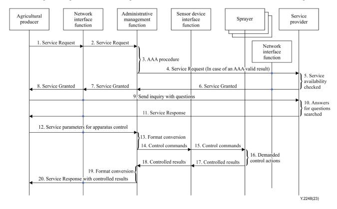
Figure 7 – Information flow for service-provider-aided control
