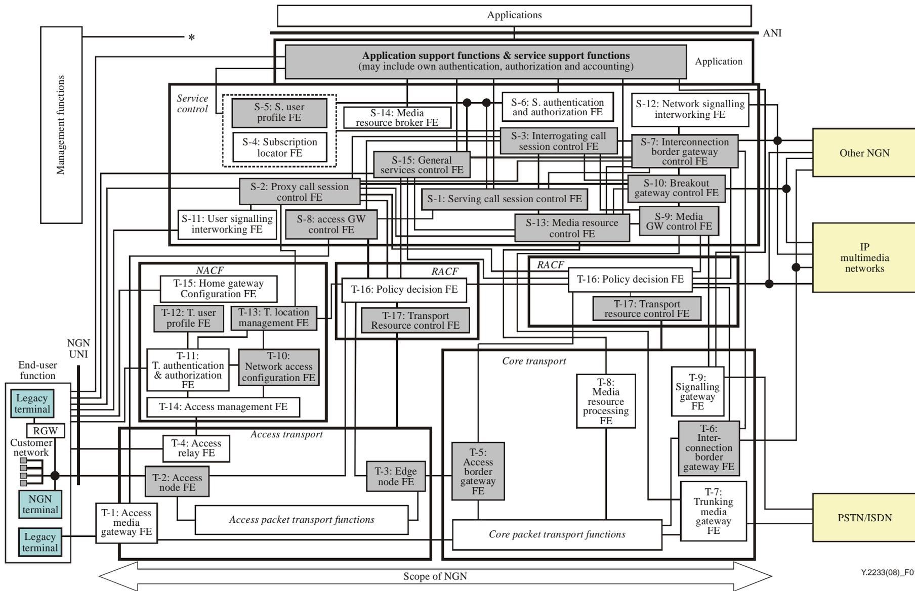
Figure 1 – Positioning of accounting and charging functions in the NGN functional architecture for release 1
