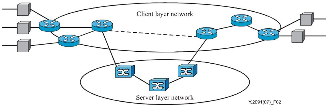
**Figure 2 – Illustration of client and server layer networks**
