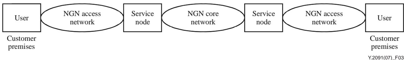
**Figure 3 – General horizontal components**
