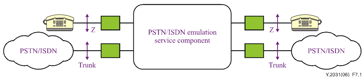
Figure 7-1 – Legacy configurations supported by IMS-based PES
