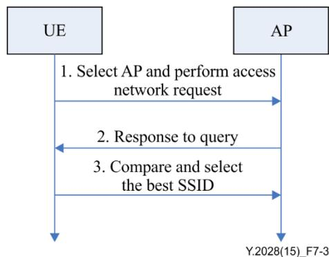
**Figure 7-3 – Terminal-based access discovery**
