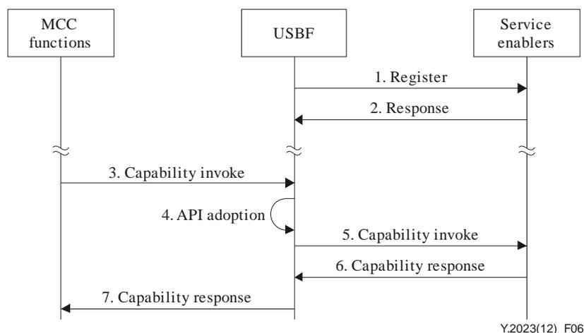
**Figure 6 – Procedure to use USBF**
