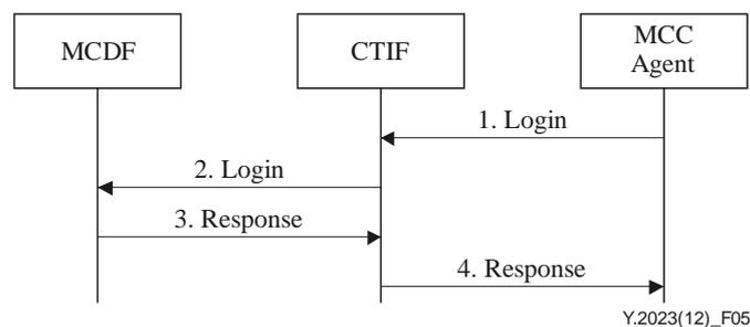
**Figure 5 – MCC service initialization procedure**
