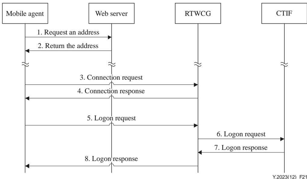
**Figure 21 – Procedure for supporting the mobile agent**
