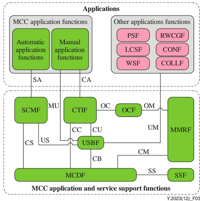
**Figure 3 – Logical diagram and reference points in the MCC**
