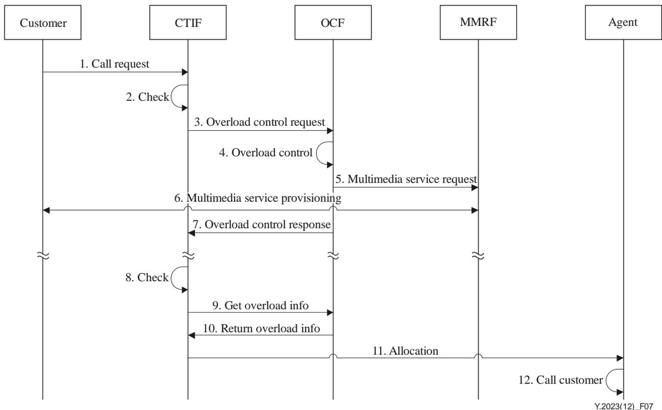
**Figure 7 – Overload control procedure**
