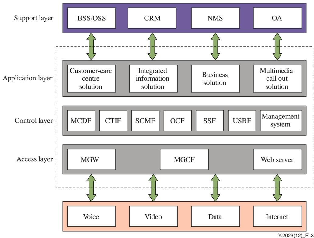
**Figure I.3 – MCC layered architecture**
