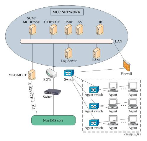
Figure I.1 – Deployment for a non-IMS network
