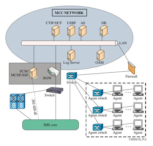
**Figure I.2 – Deployment for an IMS network**
