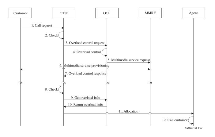
Figure 7 – Overload control procedure
