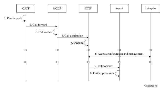
Figure 4 – Queuing and distribution procedure of communication requests
