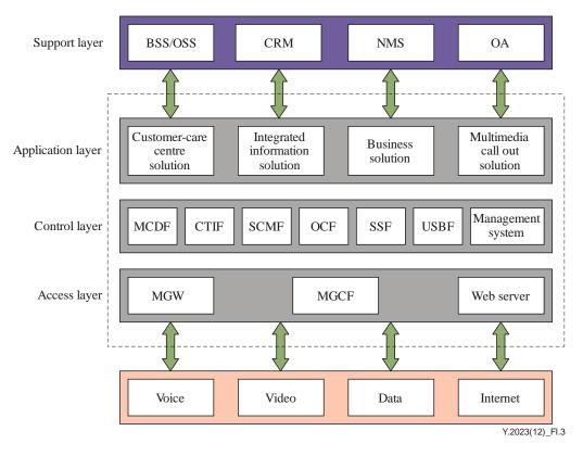
Figure I.3 – MCC layered architecture
