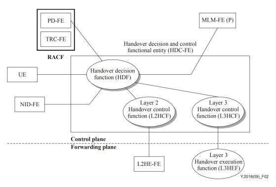
Figure 2 – Relations of HDC-FE sub-functions
