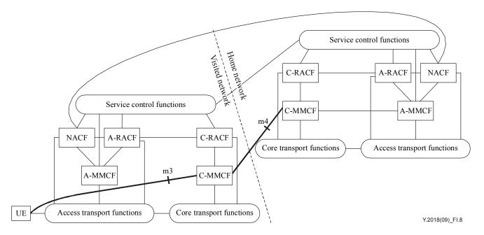
Figure I.8 – Roaming architecture for host-based mobility using m3 and m4
