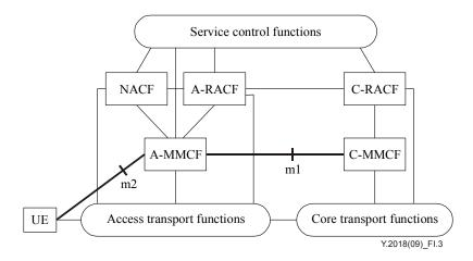
Figure I.3 – Non-roaming architecture for host-based mobility using m1 and m2
