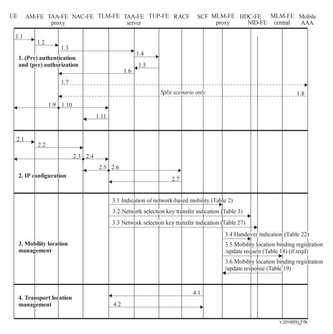
Figure 6 – Information flows for attachment, case of network-based mobility
