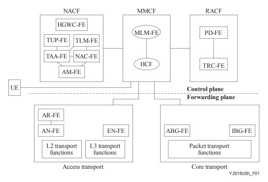
Figure 1 – Position of mobility management and control in the NGN transport stratum architecture
