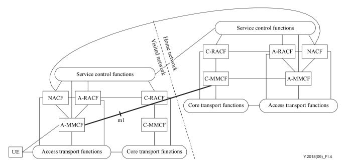
Figure I.4 – Roaming architecture for network-based mobility using m1
