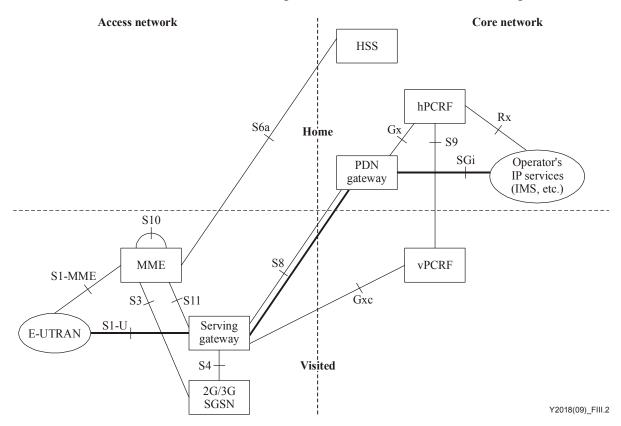
Figure III.2 – Roaming architecture for 3GPP accesses within EPS using PMIP-based S8
