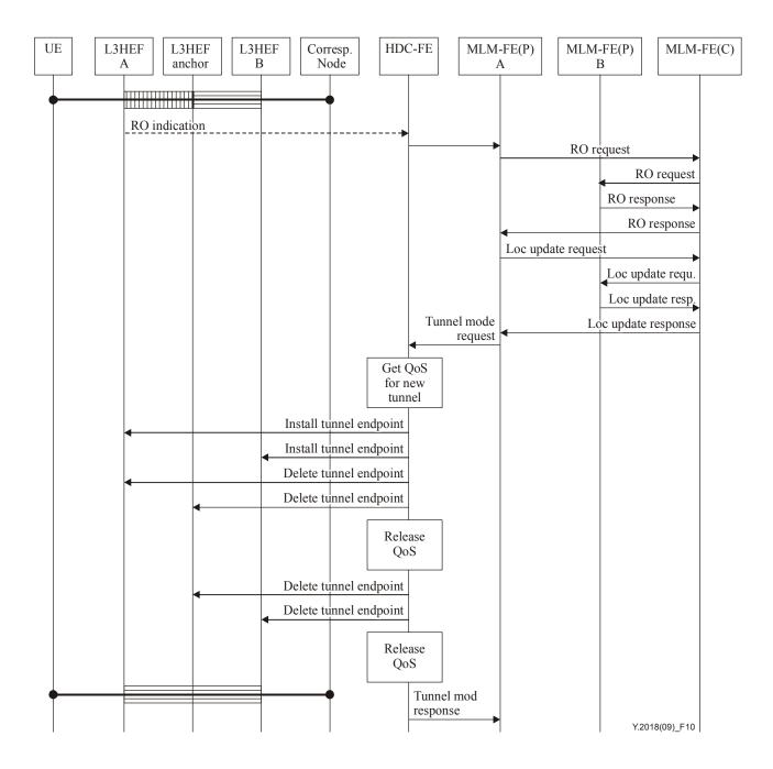
Figure 10 – Routing optimization assuming network-based mobility at each end
