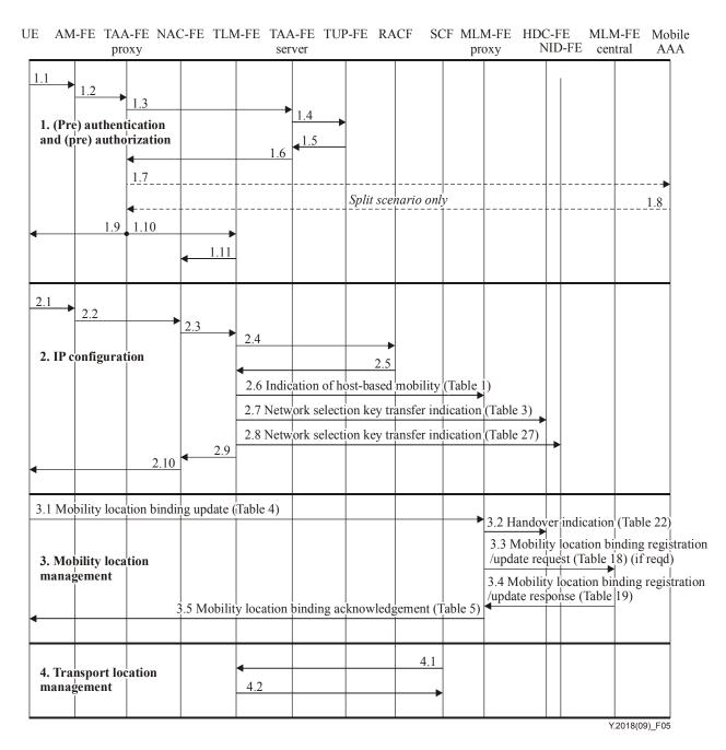
Figure 5 – Information flows for attachment in the case of host-based mobility
