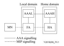
**Figure II.1 – MIPv4 architecture according to the IETF**
