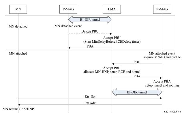
Figure II.3 – PMIPv6 signalling flows for handover
