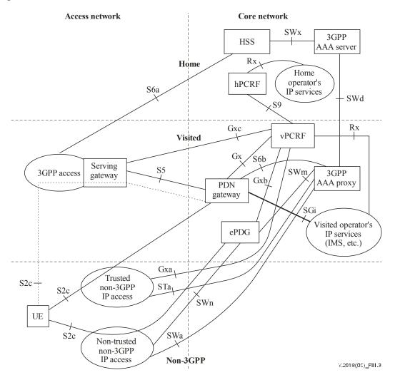
Figure III.3 – Roaming architecture for EPS using S5, S2c – Local breakout
