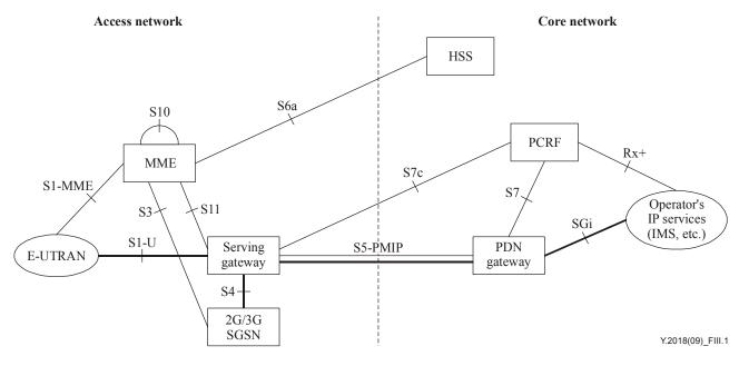
Figure III.1 – Non-roaming architecture for 3GPP accesses within EPS using PMIP-based S5
