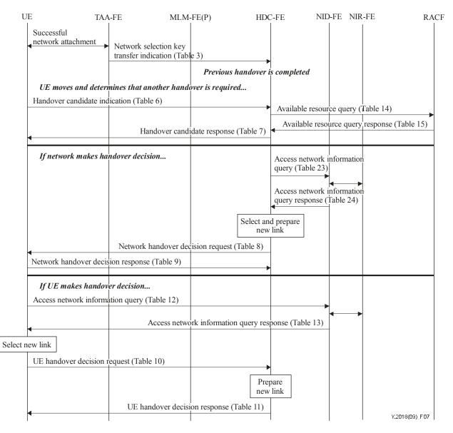
Figure 7 – Illustration of network discovery and decision procedure – Network-triggered handover
