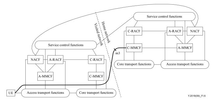
Figure I.6 – Roaming architecture for host-based mobility using m3
