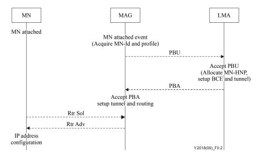
Figure II.2 – Signalling flows for PMIPv6 initial attachment
