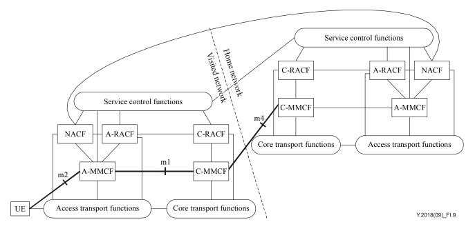
Figure I.9 – Roaming architecture for host-based mobility using m1, m2 and m4
