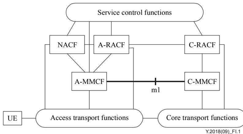
**Figure I.1 – Non-roaming architecture for network-based mobility using m1**
