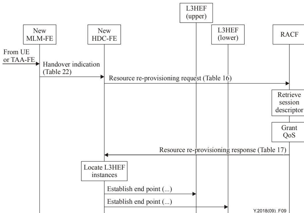
Figure 9 – Procedure for establishing a new layer 3 path
