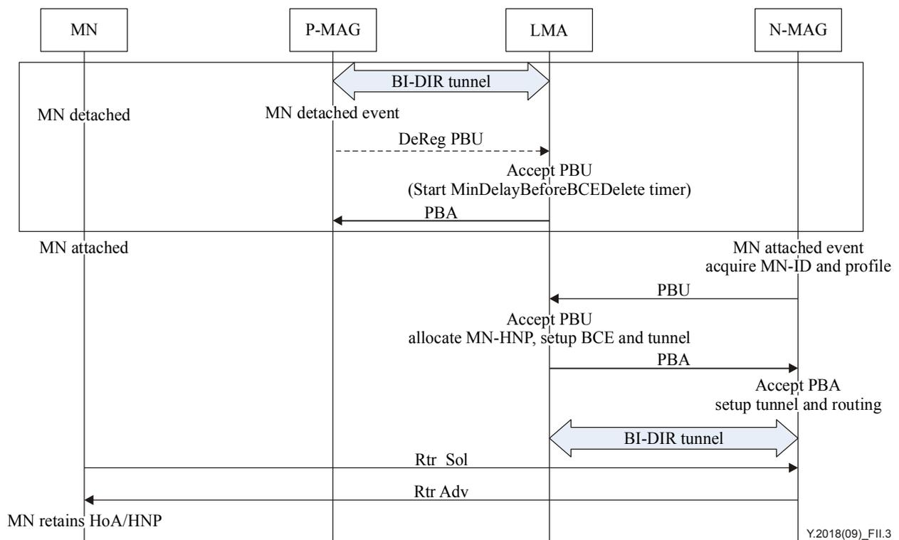
**Figure II.3 – PMIPv6 signalling flows for handover**
