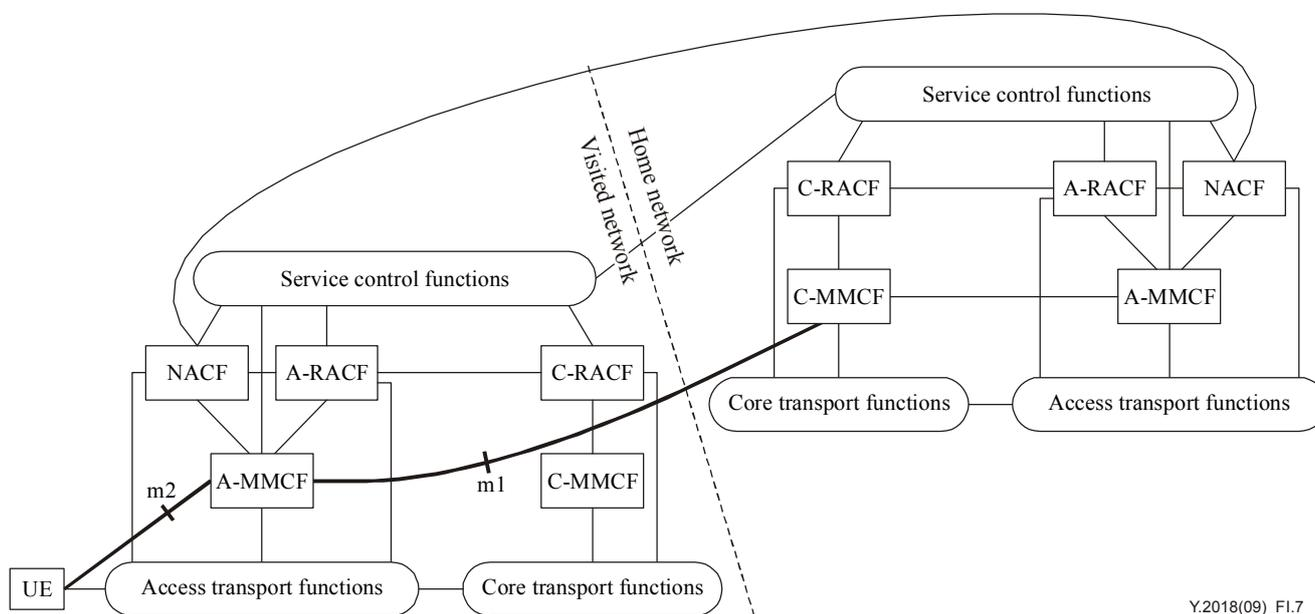
**Figure I.7 – Roaming architecture for host-based mobility using m1 and m2**
