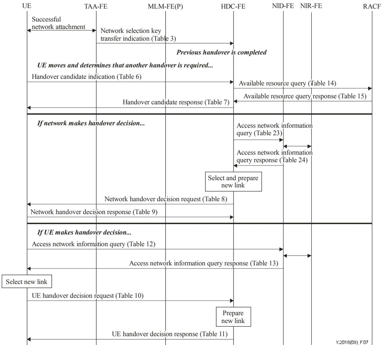
**Figure 7 – Illustration of network discovery and decision procedure – Network-triggered handover**
