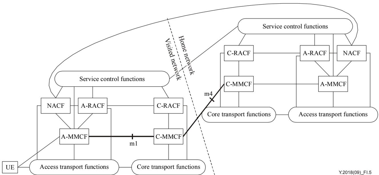
**Figure I.5 – Roaming architecture for network-based mobility using m1 and m4**
