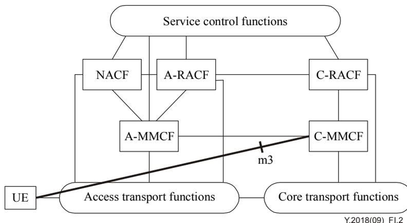
**Figure I.2 – Non-roaming architecture for host-based mobility using m3**
