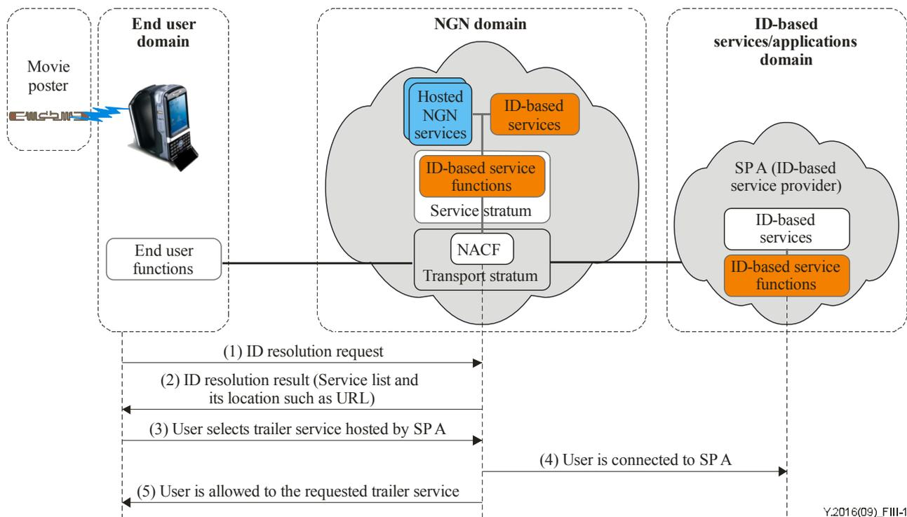
**Figure III.1 – Typical ID-based application and services information flow**
