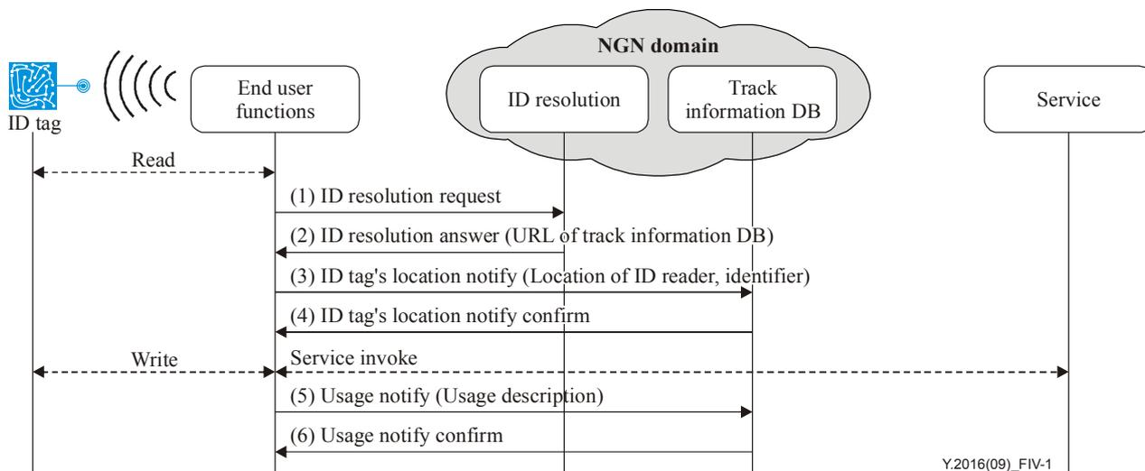
**Figure IV.1 – Example of information flows for object traceability and usage traceability**
