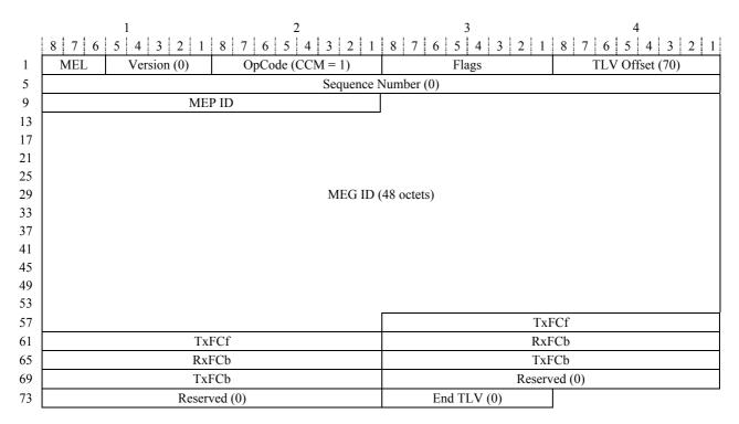
Figure 9.2-1/Y.1731 – CCM PDU format
