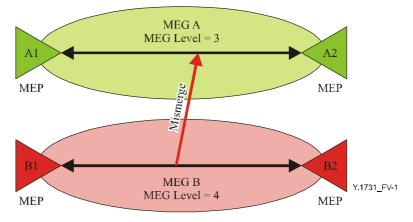
No defects detected as no mismerge exists to MEG B
