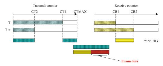
Figure III.2/Y.1731 – Transmit Counter wraps around
