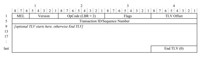
Figure 9.4-1/Y.1731 – LBR PDU format
