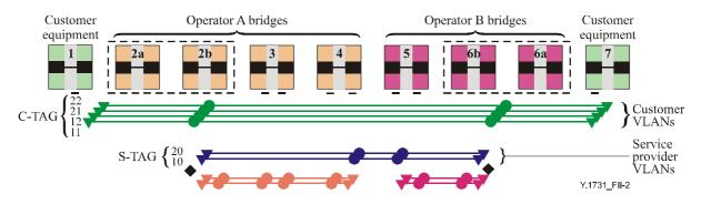
Figure II.2/Y.1731 – Example MEG level assignment for independent MEG levels
