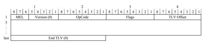
Figure 9.1-1/Y.1731 – Common OAM PDU format
