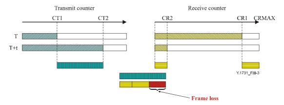
Figure III.3/Y.1731 – Receive Counter wraps around
