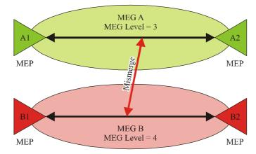
No defects detected by MEPs of MEG A as only MEG Levels 3 and lower are considered.
