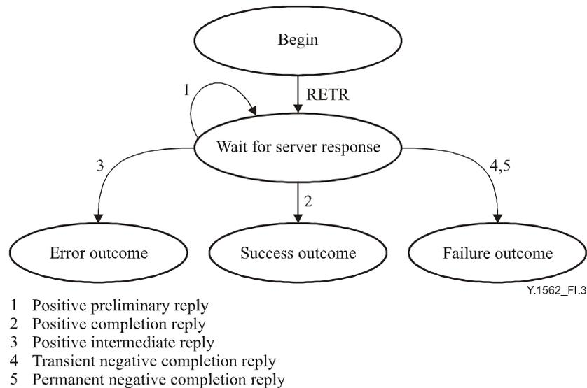
**Figure I.3 – State diagram for the RETR command (from IETF RFC 959)**
