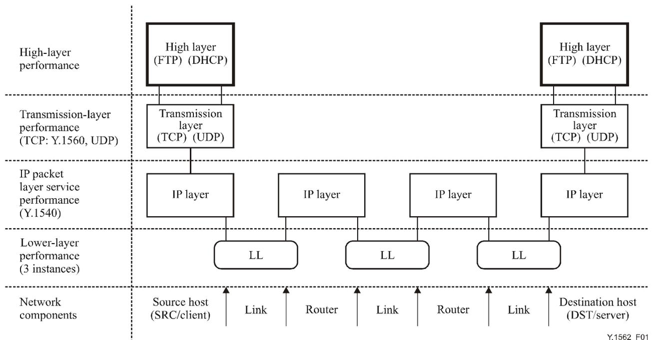
**Figure 6-1 – Layered model for higher layer – Example**
