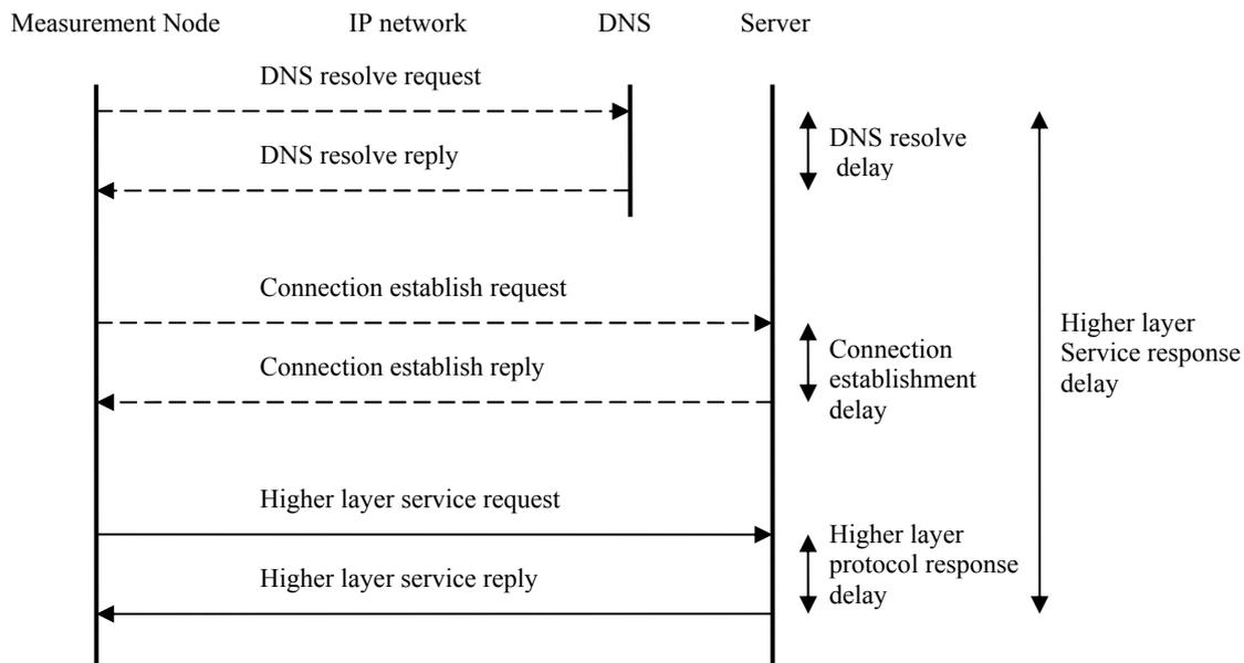
**Figure 7-1 – Higher-layer service response delays**
